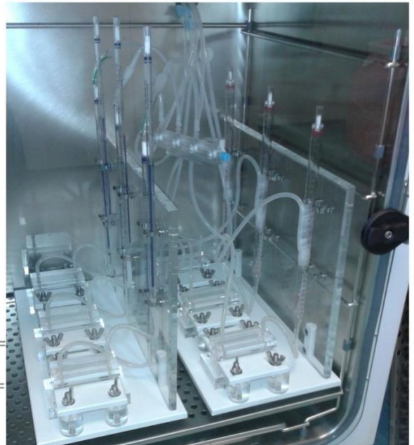
Figure 2.1 Schematic diagram of in-house parallel plate flow chambers.
