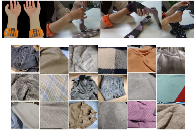
Fig. 1: Top - Left to right: Sensor placement for our FabricTouch dataset; examples from Phase II collection showing assessment of smoothness (finger caress), warmth (hand inside sock), and flexibility (pulling opposite side) respectively. Bottom - Examples of garments from Phase I collection.
