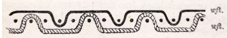
Figure 8.09 Double weave diagram with warp strings in line, as on the loom (Ashenhurst, 1892 p. 17)
