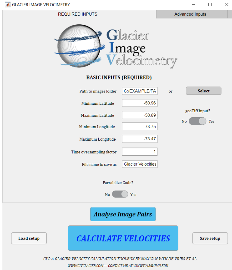
Fig. 4.6 GIV GUI main window with options to set the path to the images folder, add minimum and maximum latitude/longitude values (not required for geotiff input), set the time oversampling factor and 'Analyze image Pairs' (which calculates the 'Total number of image pairs' and the 'Number of image pairs per individual oversample')
