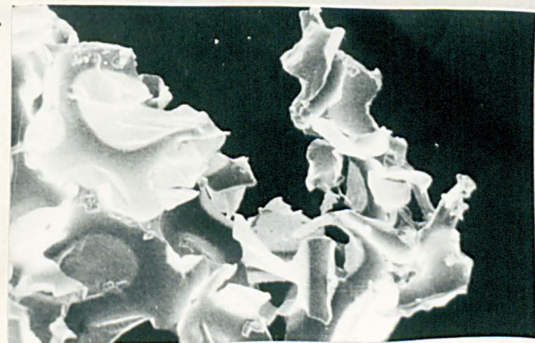
Polyester fibre reinforced foam 75\text{kgm}^{-3} (treated with Kenreact KRTTS titanate. Magnification 150x.
