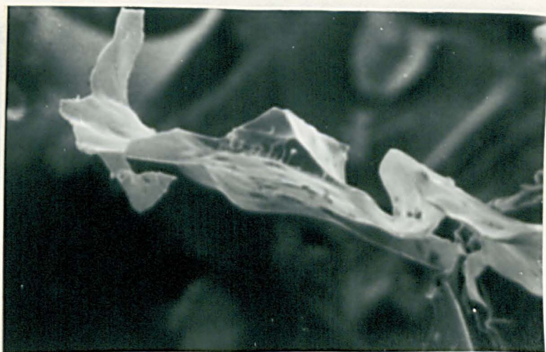
Polyester fibre reinforced foam 101\text{kgm}^{-3} . Magnification 197x.
