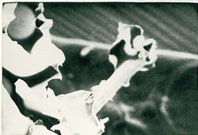
Glass fibre reinforced foam 40\text{kgm}^{-3} . Magnification 154x.
