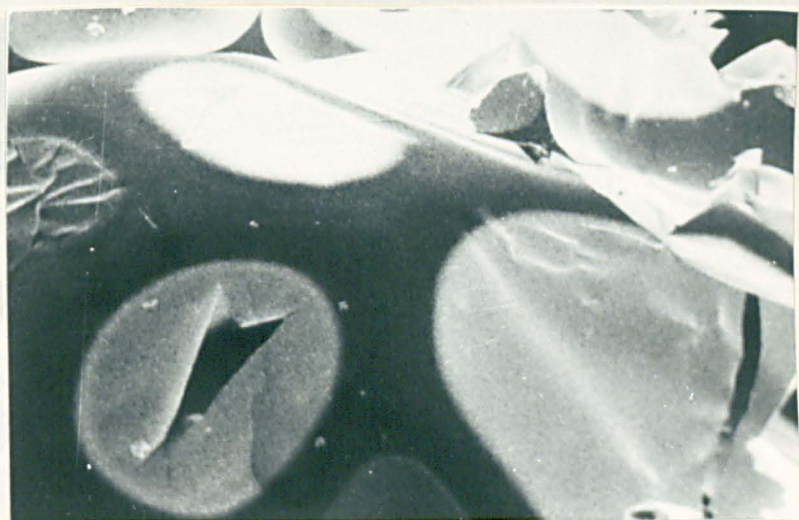
Unreinforced foam 142\text{kgm}^{-3} . Magnification 1877x.
