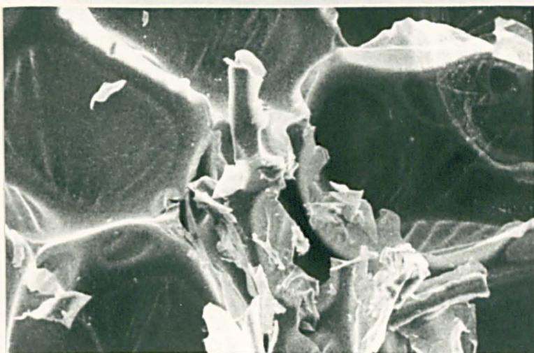
Polyester fibre reinforced foam 67\text{kgm}^{-3} . (treated with Kenreact titanate KR44). Magnification 149x.
