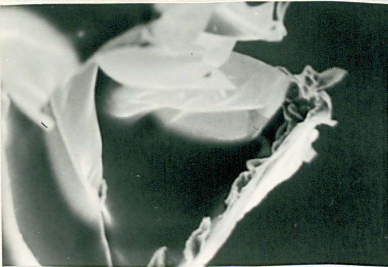
Glass fibre reinforced foam 80\text{kgm}^{-3} . Magnification 221x.
