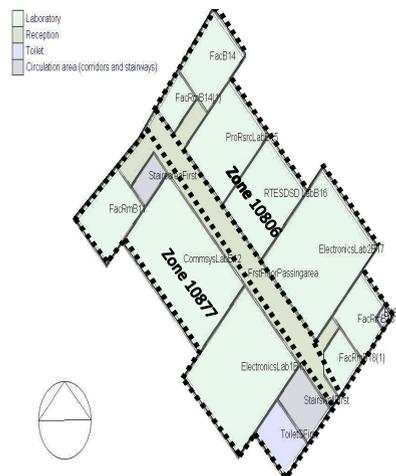
FIGURE 2. Zone structure of the first floor.
