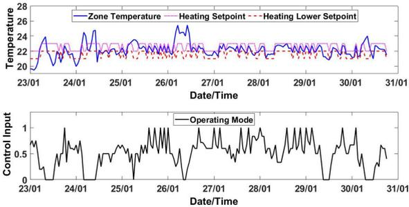
FIGURE 16. Air temperature of Zone3539 maintained by ON/OFF control at PMV-based setpoints.
