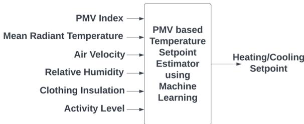
FIGURE 5. PMV-based temperature setpoint estimator using ML.
