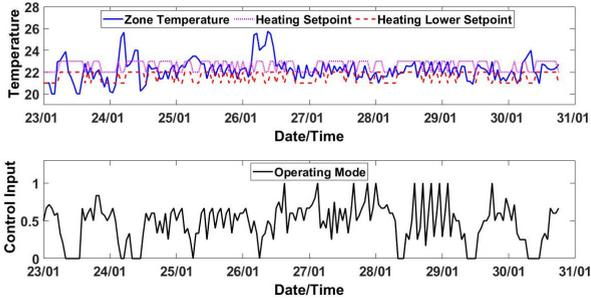
FIGURE 14. Air temperature of Zone3539 maintained by the MPC at the PMV-based setpoints during Winter Season.
