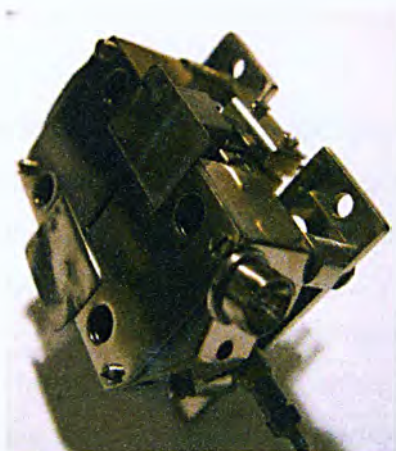
Figure 6.31 The more sophisticated design of the EI source suitable for low energy ion beams, including advanced electron trap for reducing secondary emission.
