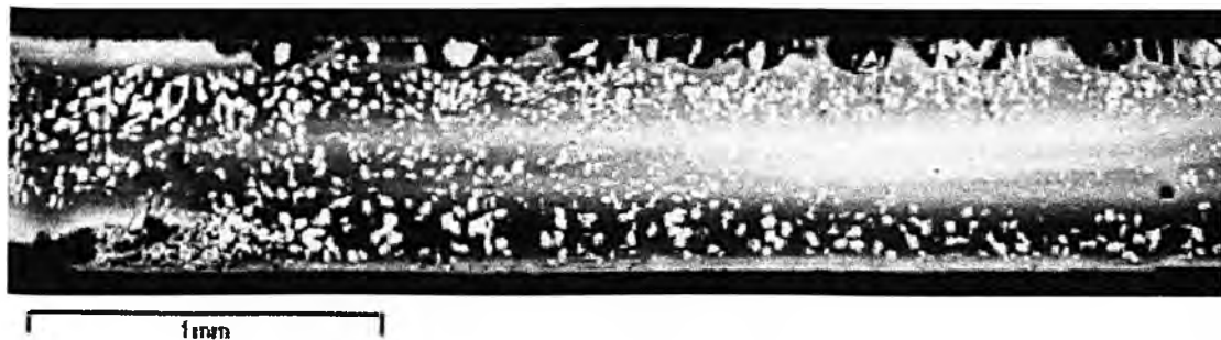
Figure 7.1 SEM image of an unconditioned Re filament loaded with Sr in HCl.
