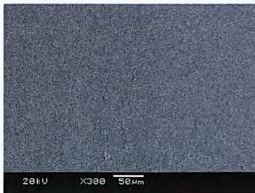
Figure 7.6 Topographic image of a Re filament baked at \sim 1140^{\circ}\text{C} .
