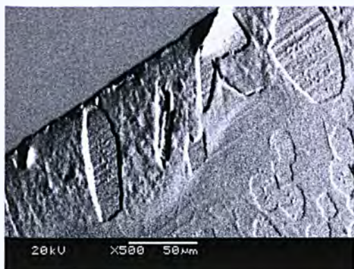
Figure 7.5 Topographic image of an unconditioned Re filament.
