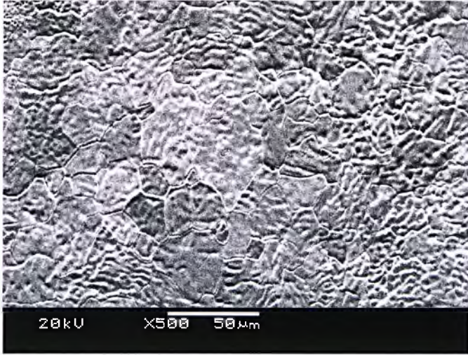
Figure 7.7 Carburized rhenium filament and the formation of large grains.
