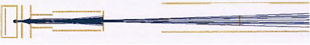
Figure 6.33 SIMION ion optics bench for the EI source. Red marks show the position where the phase space of the ions is determined.
