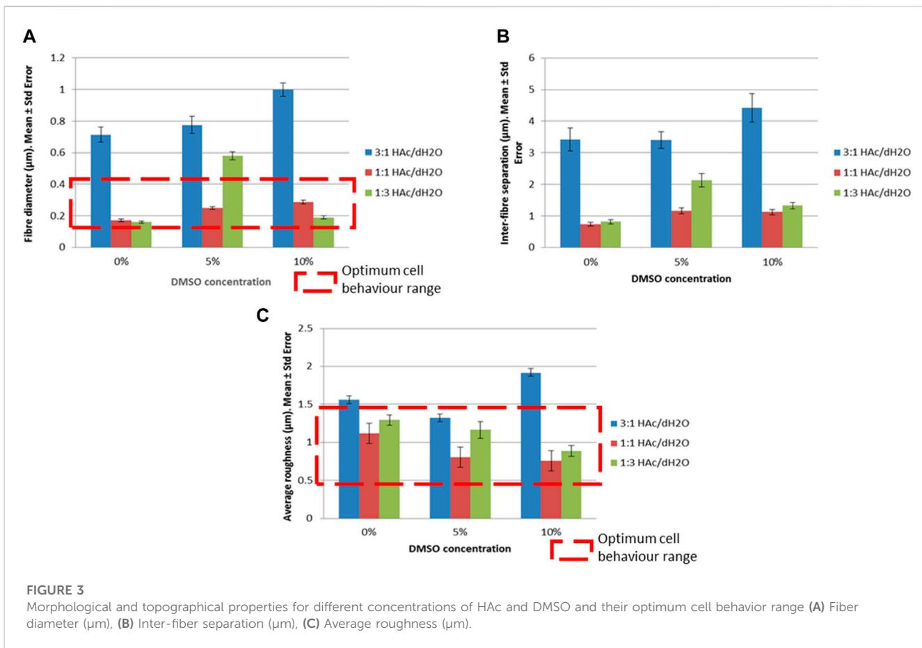
**FIGURE 3** Morphological and topographical properties for different concentrations of HAC and DMSO and their optimum cell behavior range (A) Fiber diameter (µm), (B) Inter-fiber separation (µm), (C) Average roughness (µm).
