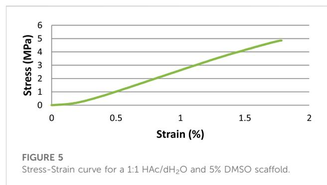
straighten in the direction of the applied load and recover their structure once load has been removed, a linear region where the Young's modulus was calculated for each sample, and the yield region. A typical stress-strain curve shown in Figure 5.
