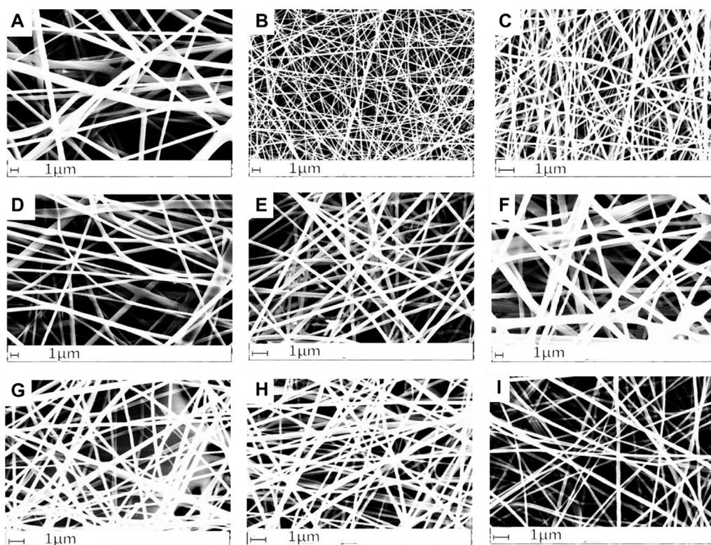
**FIGURE 2** Electrospun scaffold obtained with a concentration of gelatin 25% w/v dissolved in concentrations (A) 3:1 HAC/dH<sub>2</sub>O and 0% DMSO, (B) 1:1 HAC/dH<sub>2</sub>O and 0% DMSO, (C) 1:3 HAC/dH<sub>2</sub>O and 0% DMSO, (D) 3:1 HAC/dH<sub>2</sub>O and 5% DMSO, (E) 1:1 HAC/dH<sub>2</sub>O and 5% DMSO, (F) 1:3 HAC/dH<sub>2</sub>O and 5% DMSO, (G) 3:1 HAC/dH<sub>2</sub>O and 10% DMSO, (H) 1:1 HAC/dH<sub>2</sub>O and 10% DMSO, (I) 1:3 HAC/dH<sub>2</sub>O and 10% DMSO.
