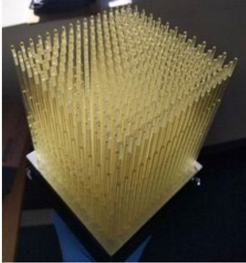
Figure 30: Test swabs manufactured on a Formlabs 3D Printer (Source: (Formlabs, 2020) (permission granted))
