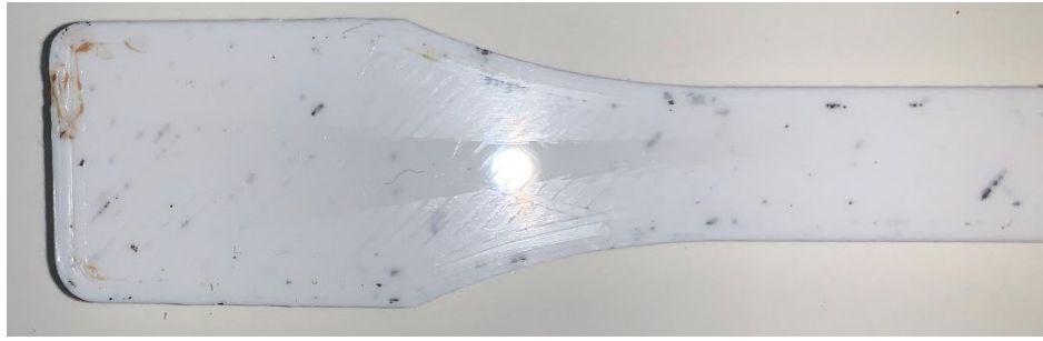
Figure 26: Burning and discolouration of sample 21C which appears to be randomly occurring
