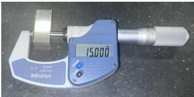
Figure 48: 15mm slip gauge block measured with a micrometer
