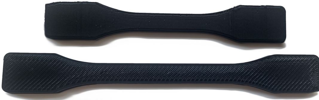
Figure 68: Images of dog bone samples (top: vertical printing orientation, bottom: horizontal printing orientation)
