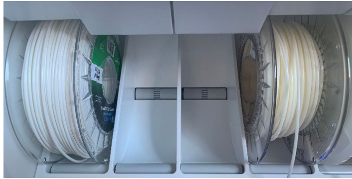
Figure 21: A visual comparison of the colour difference between PLA-N Signal White (left) and PLA-N Natural (right)
