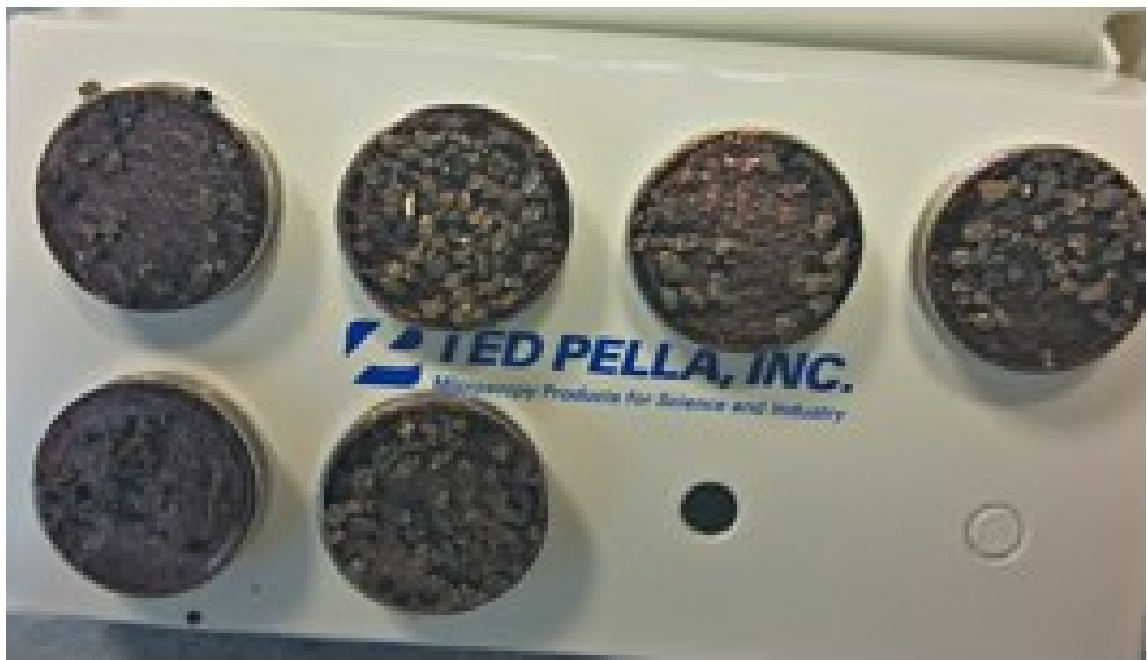
SI 4.1: ABDite® bioparticles coated with thin layer of gold mounted on studs for SEM analysis.
