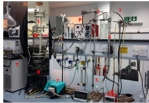
Fig.1 Picture of the lab-scale expanded bed bioreactor (1 - Expanded bed column, 2 - Recycle, 3 - Outlet, 4 - recirculation column, 5 - \text{N}_2 gas inlet, 6 - Feed pump, 7 - Fluidizing pump, P - pH sensor, R - refuse bag T - Temperature sensor, W - Water jacket).
