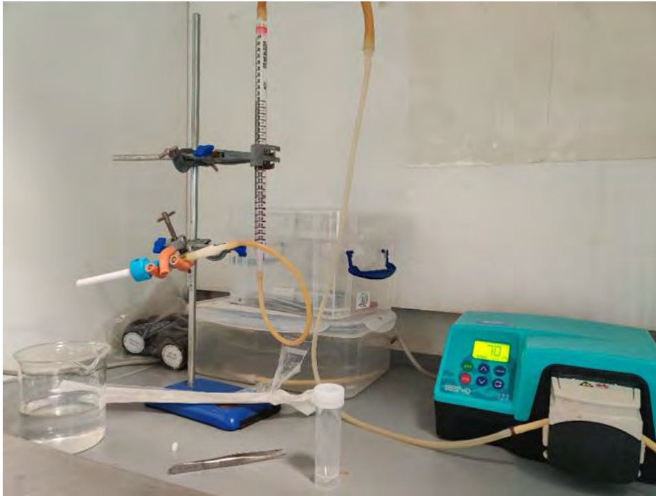
Figure 8: Setup for the collection of cigarette smoke extract. Retort stand, tubing, stripette, and pump were set up with a Marlboro Gold cigarette to collect CSE-infused media for cell treatment.
