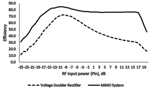
Fig. 3: Efficiency comparison of the voltage doubler rectifier and the MIMO design.
