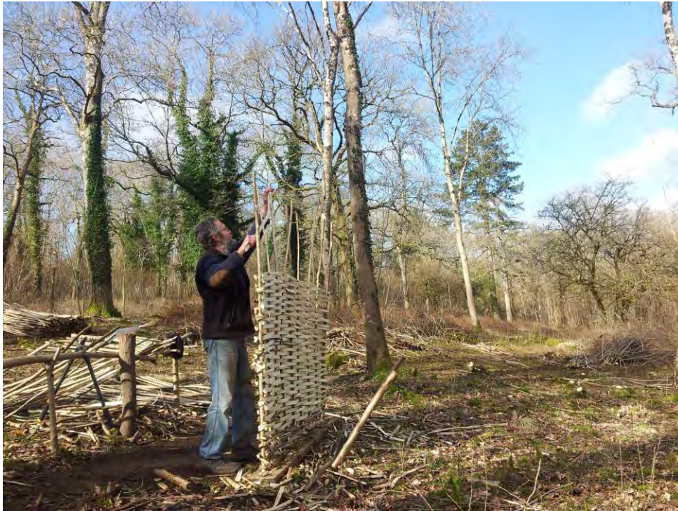
Figure 17. Don Taylor, Hurdle-Maker constructs a hazel hurdle from the coppice he has recently cut, a process followed by successive generations of coppice-workers for at least 500 years in the Chase woods. Rushmore, Wiltshire, April 2014.
