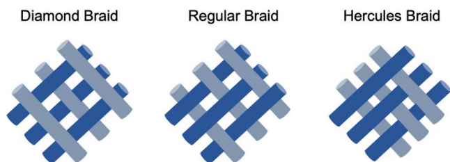
Figure 8. Three common tubular 2D braids. Diamond braid has the maximum interlacing density with a 1/1 intersection repeat (the yarn is continuously passing over one and then under one yarn). Regular braid with a 2/2 and Hercules braid with a 3/3 yarn passing. The particular braid pattern is determined by the machine set-up.
