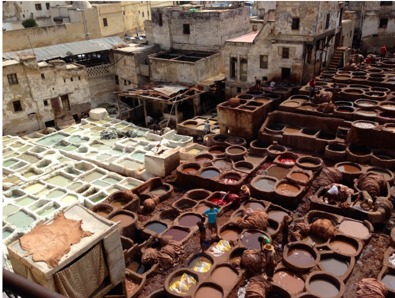
Figure 5: An example of leather processing taking place at Chouara tannery in Fez, Morocco. This is the largest tannery in the city and has continued to use only manual labour since medieval times (Patowary, 2014). These traditional techniques offer inadequate protection from toxic chemicals to workers' health and the environment. Photo credit: (Nash, 2014) Photo credit: 'Fes Morocco Tannery - sept 2014 - 04' by andynash, licensed under CC BY-sA 2.0. To view a copy of this license, visit https://creativecommons.org/licenses/by-sa/2.0/?ref=openverse .
