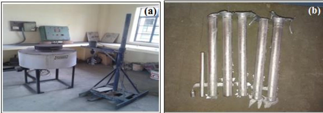
Figure 1. (a) Electrical melting furnace with mechanical stirrer (b) cylindrical castings
