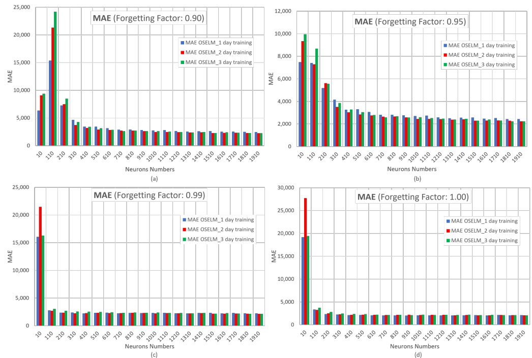
Figure 14. MAE metric for the OS-ELM network with forgetting factors at (a) 0.90, (b) 0.95, (c) 0.99, and (d) 1.00
