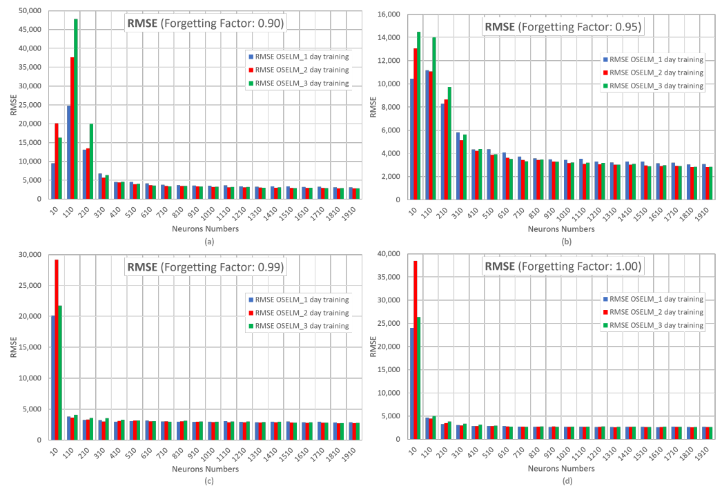
Figure 13. RMSE metric for the OS-ELM network with forgetting factors at (a) 0.90, (b) 0.95, (c) 0.99, and (d) 1.00.
