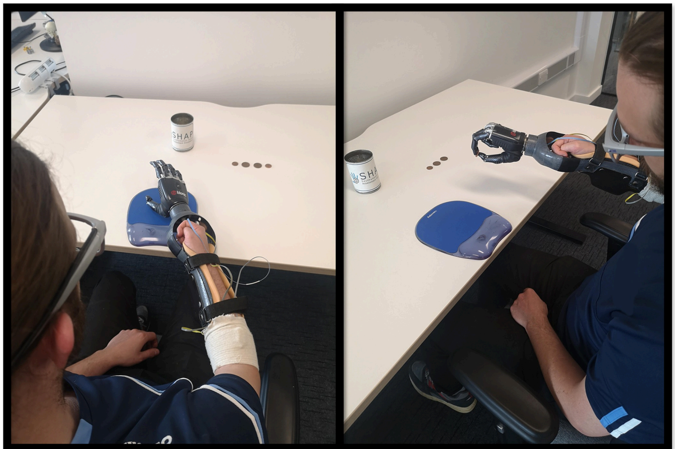
Fig 1. Showing the coin task setup (left) and the participant reaching to drop a coin into the jar (right).
