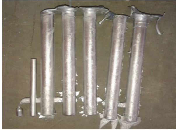
2 Figure 1. Die cast Al-15Si-4Ni-2Cu alloy
