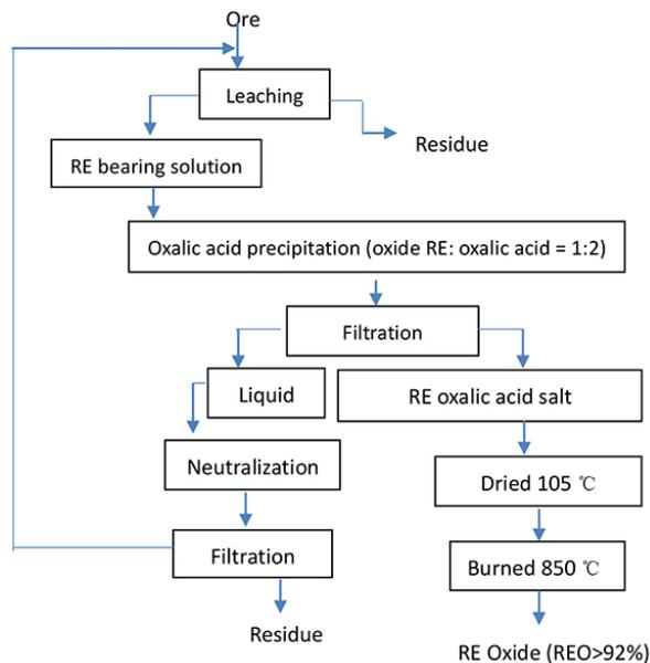
Figure 5—REE extraction technique for weathered crust elution deposit REE ore
