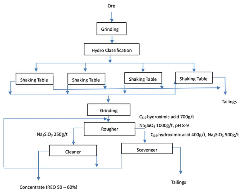
Figure 3—Gravity separation–flotation process at Mianning REE mine
