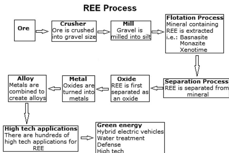
Figure 1—Conventional REE processing technology and REE applications
