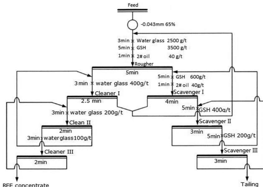
Figure 6—Flotation flow sheet for Maoniuping REE ore
