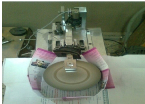
9 10 Figure 1. Dry sliding Pin on Disc type wear testing machine
