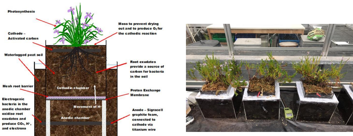
Figure 3 - Old fuel cell design on the left and constructed fuel cell with the old design on the right containing peat and heather.
