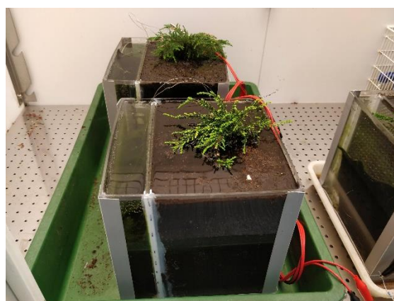
Figure 5 - New fuel cell design containing Calluna vulgaris in peat soil in the right chamber and the cathode filled with water in the left chamber.
