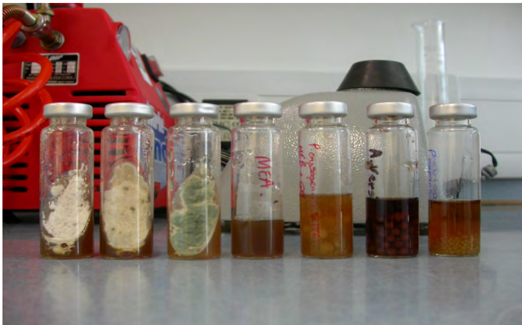
Fig.81. Vials containing samples for use with the Gas chromatography- Mass spectrometry for Solid Phase Micro Extraction- Head Space (SPME) Analysis. The three vials on the left contain fungal cultures grown on MEA slopes. The vial in the middle is un-inoculated MEA only and the three on the right are fungal cultures which have been grown in broth culture (MEA and gelatine) and transferred into the vials. Film strips in the GC vials are not included.
