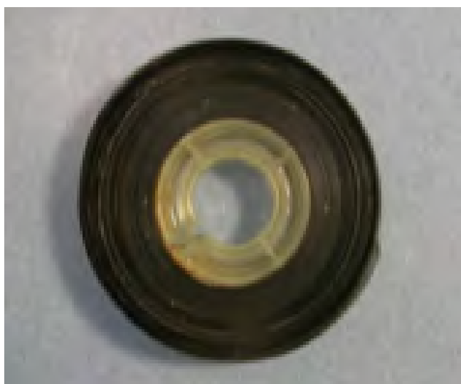
Fig.25. RR1399 after Test 1 and Test 2 before the laminectomy was performed. Most of the mould growth appears to have been removed by the physical winding of the film reel.
