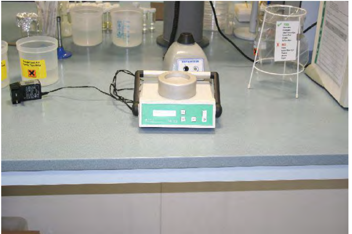
Fig.17. Air Sampler GS100 used for sampling with variable control up to 100L 3 .
