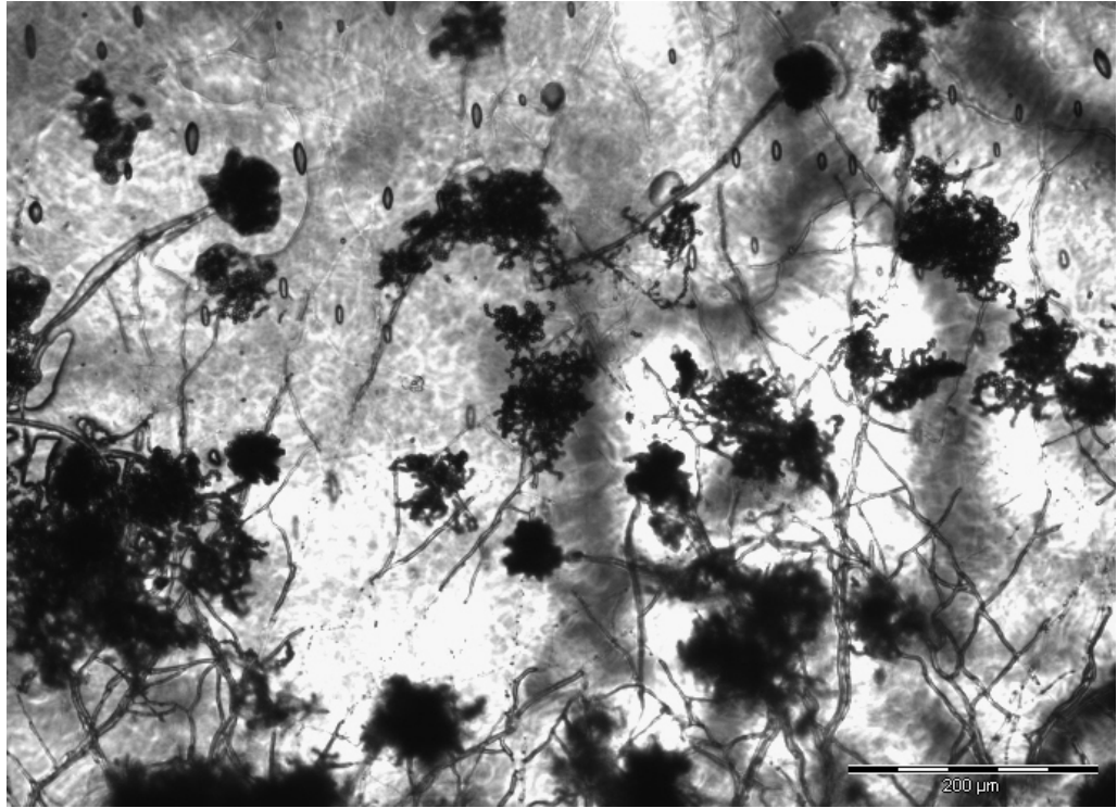
Fig.57. Image of the edge of the cellulose acetate under light microscope (x10) which has been separated from the emulsion layer, during the process of removal from the agar plate from method 2. Aspergillus conidiophores and mycelia can be seen.
