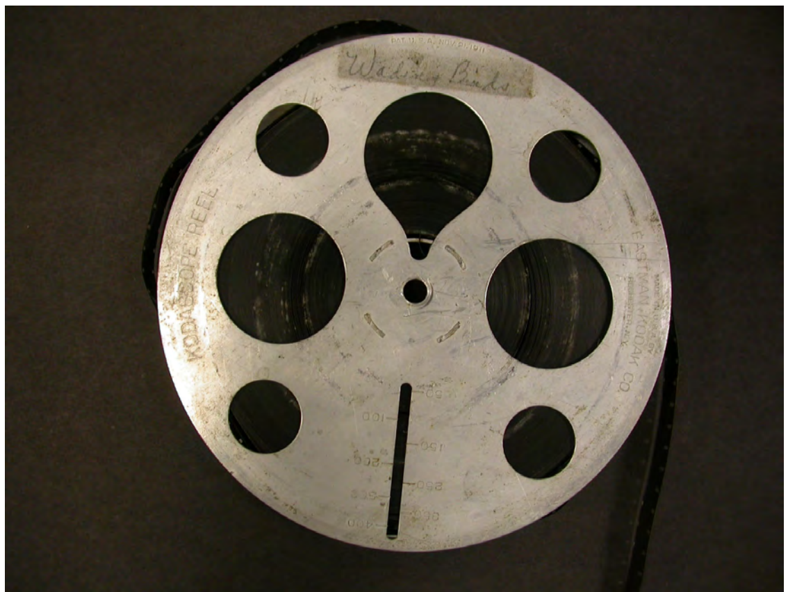
Fig.12. Category 2 - a dusty appearance and a few white spots may be visible but no clearly visible mycelial growth.
