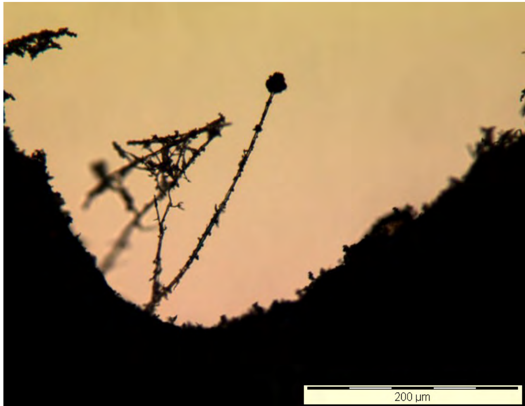
Fig.50. Light microscopy image (x40) of reel RR1399 show showing the presence of an Aspergillus conidiophore. This reel was heavily contaminated and high number of CFUs were isolated from air sampling. The predominant coloniser of this reel was A.versicolor .
