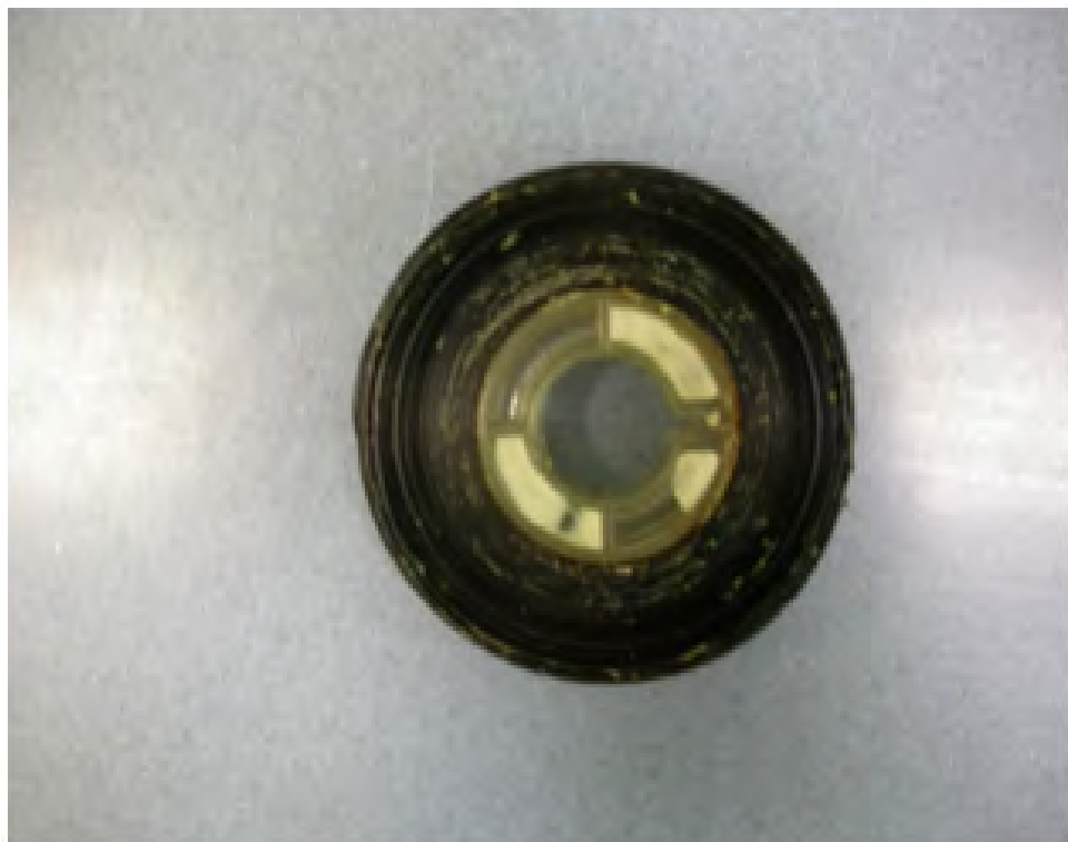
Fig.22. Reel RR1399 which has been covered in art masking fluid (laminectomy) and allowed to air dry.
