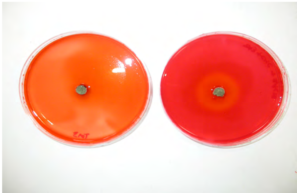
Fig.45. CMC selective agar plates with a plug of A.versicolor in the centre incubated for 5 days at 25°C and stained with Congo red. The left plate contains Technical Agar no.3 (Oxoid) with mineral salts and peptone, and the plate on the right contains Technical Agar no.3 (Oxoid) with mineral salts and peptone with added CMC 0.2% w/v. A zone of hydrolysis can be seen around the isolate on the cellulose medium indicating that Congo red stains cellulose.
