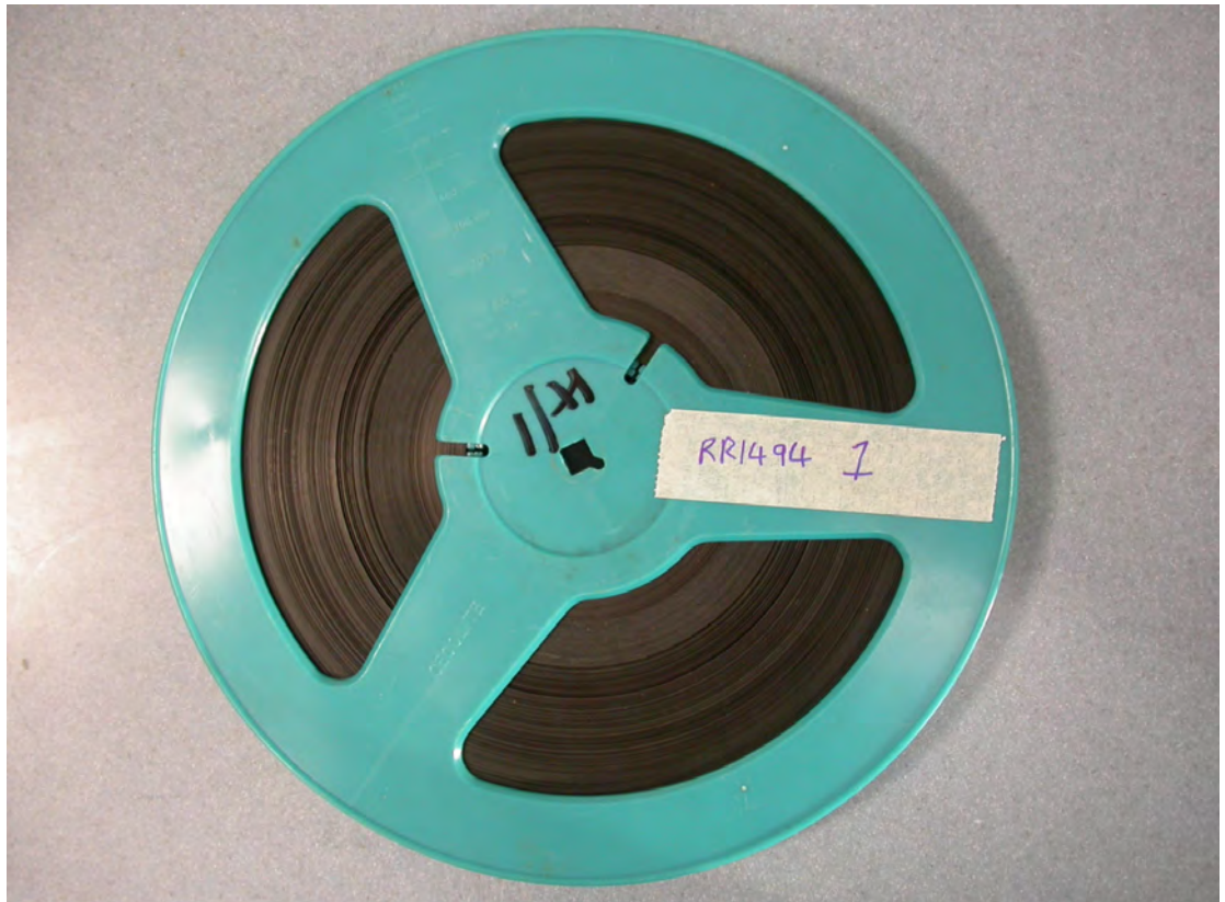
Fig.11. Category 1 - a light dust covering with no mycelial growth.
