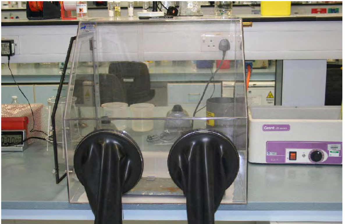
Fig.15. Isolation Glove Box (Wolf Laboratories, York, UK(Model number: 8307030 (3ft))) approximately 2.3\text{m}^3 volume) used when simulating film inspection. Access is provided via a side door (shown open on the left hand side) and rubber sleeves attached to front.
