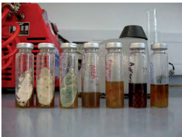
Fig. 1 Vials containing samples for use with the gas chromatography–mass spectrometry for Solid Phase MicroExtraction-HeadSpace (SPME) Analysis. The three vials on the left contain fungal cultures grown on MEA slopes. The vial in the middle is un-inoculated MEA only and the three on the right are fungal cultures which have been grown in broth culture (MEA and gelatine) and transferred into the vials.
