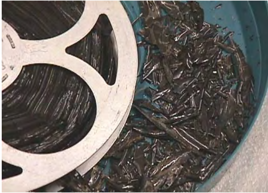
Fig.5. A cellulose acetate film reel that has been severely affected by vinegar syndrome. (Anon. (National Film and Sound Archive Australia (C), n.d.)
