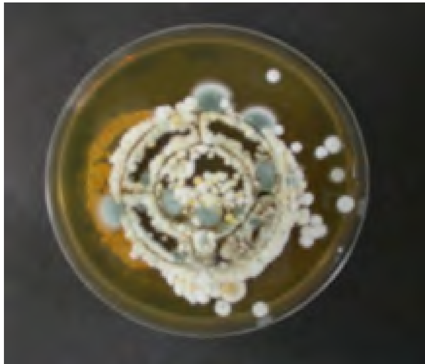
Fig.20. Pressing of the RR1399 spool resulted in heavy growth.
