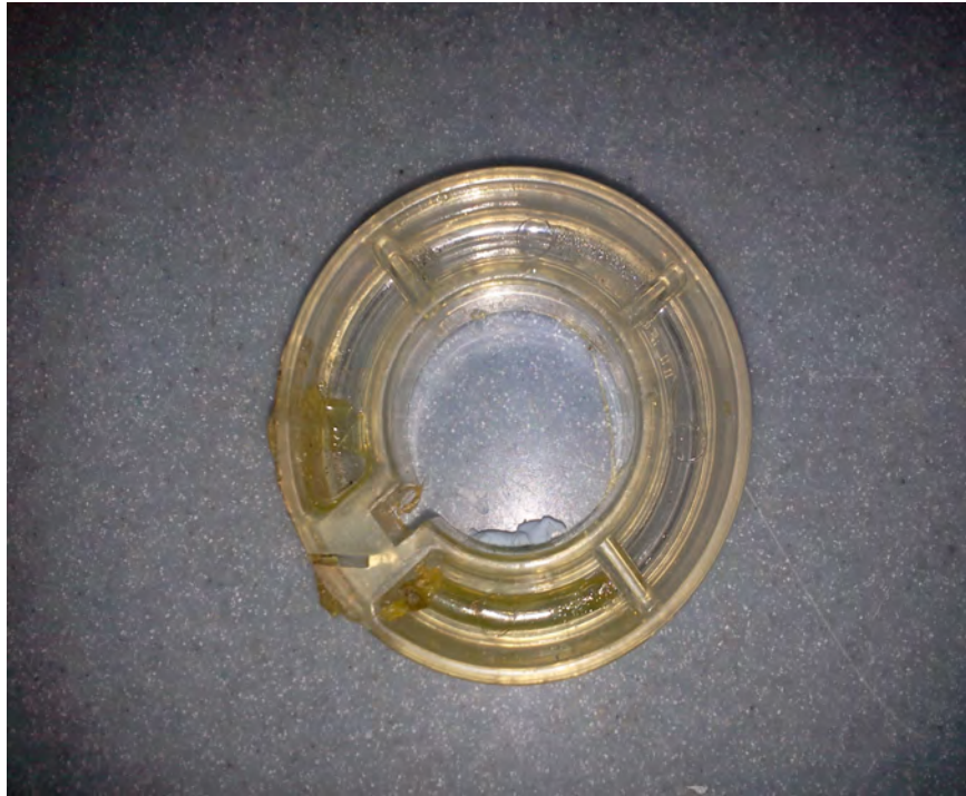
Fig 19. RR1399 spool which was cleaned with Trigene after pressing onto MEA.
