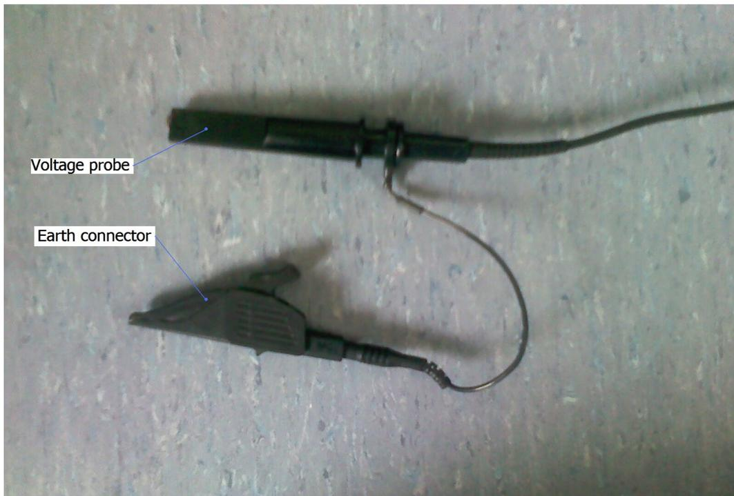
Figure 4.14: The oscilloscope voltage probe head with its earth lead.
