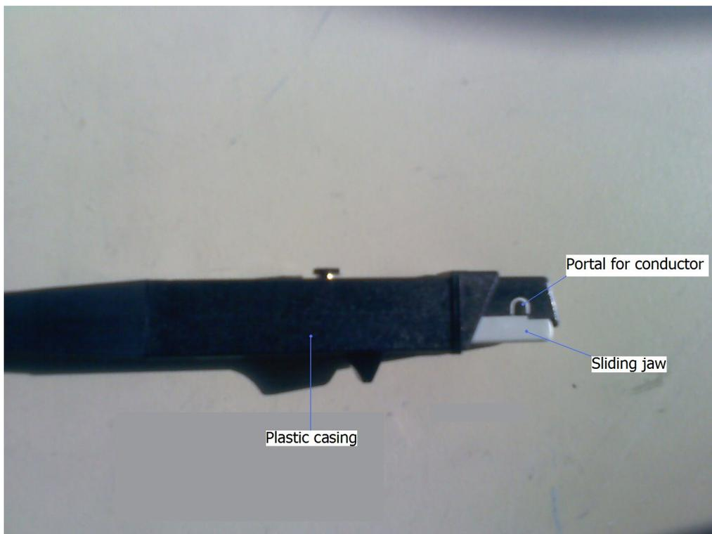
Figure 4.12: The current probe head, with labelled components.
