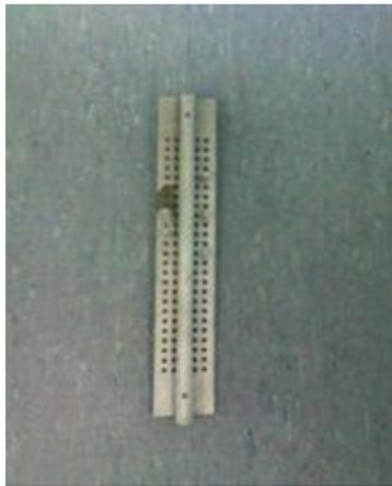
Figure 4.7: The vertical substrate holder.
