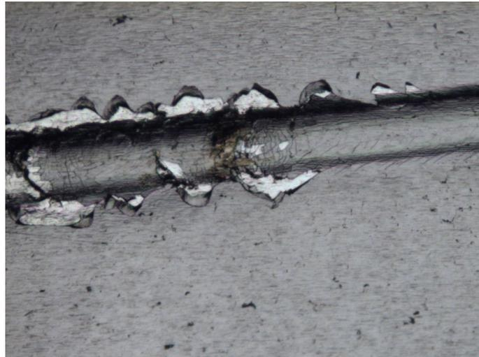
Figure 6.4: The beginning of continuous spallation around the edge of the scratch track, accompanied by intermittent spallation along the bottom of the track. Indenter motion is from right to left.
