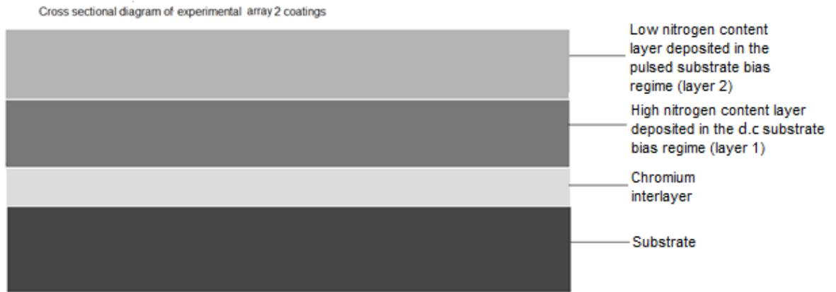
Figure 9.1: A schematic of the array 2 coatings.
