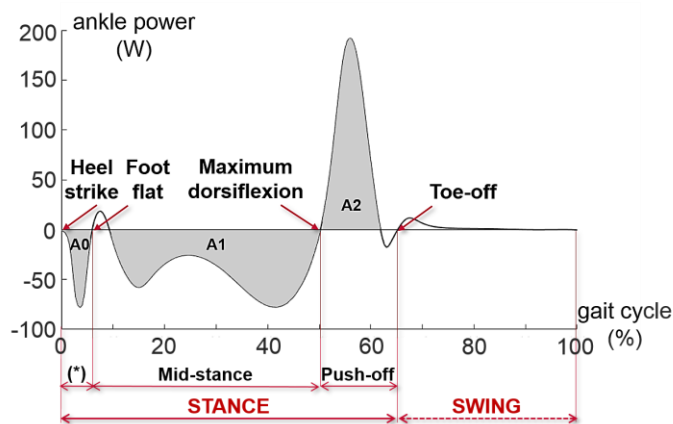
Fig. 2. Ankle power over the full gait cycle in an anatomically intact person walking at self-selected speed (data from Bari [41]). The grey areas delimited by the power curve constitute the ankle energy (work done). The negative areas – A0 and A1 – represent the negative work, that is energy absorption, while the positive area – A2 – represents the positive work that is energy generation. The symbol (*) represents the “load acceptance” phase of the gait cycle.
