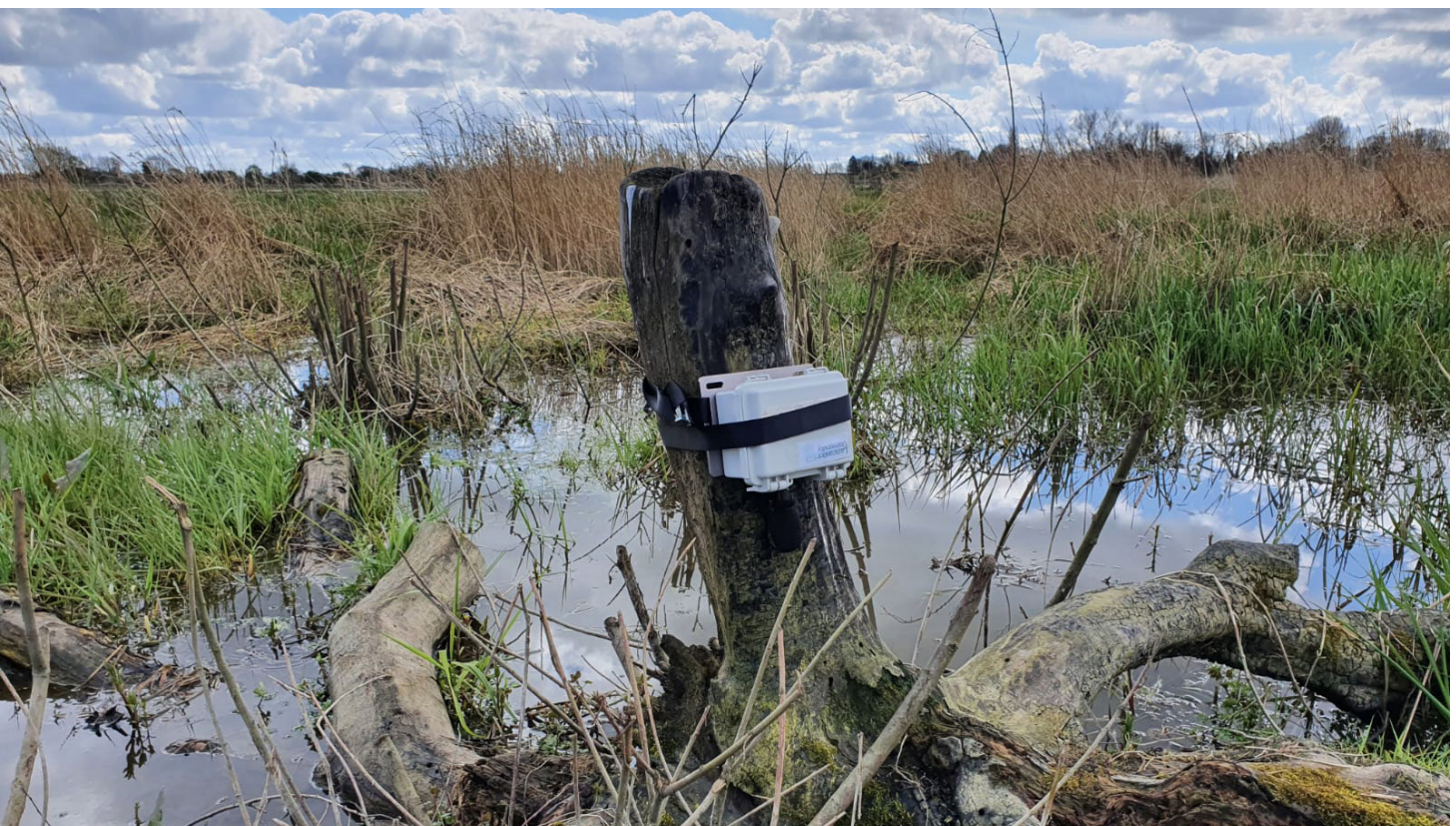
Figure 5.7. A Fronter Labs Bioacoustic Recorder deployed in a Spotted Crane Porzana porzana territory to help monitor this rare, nocturnal, and elusive wetland breeding species. Credit: Oliver Metcalf.
