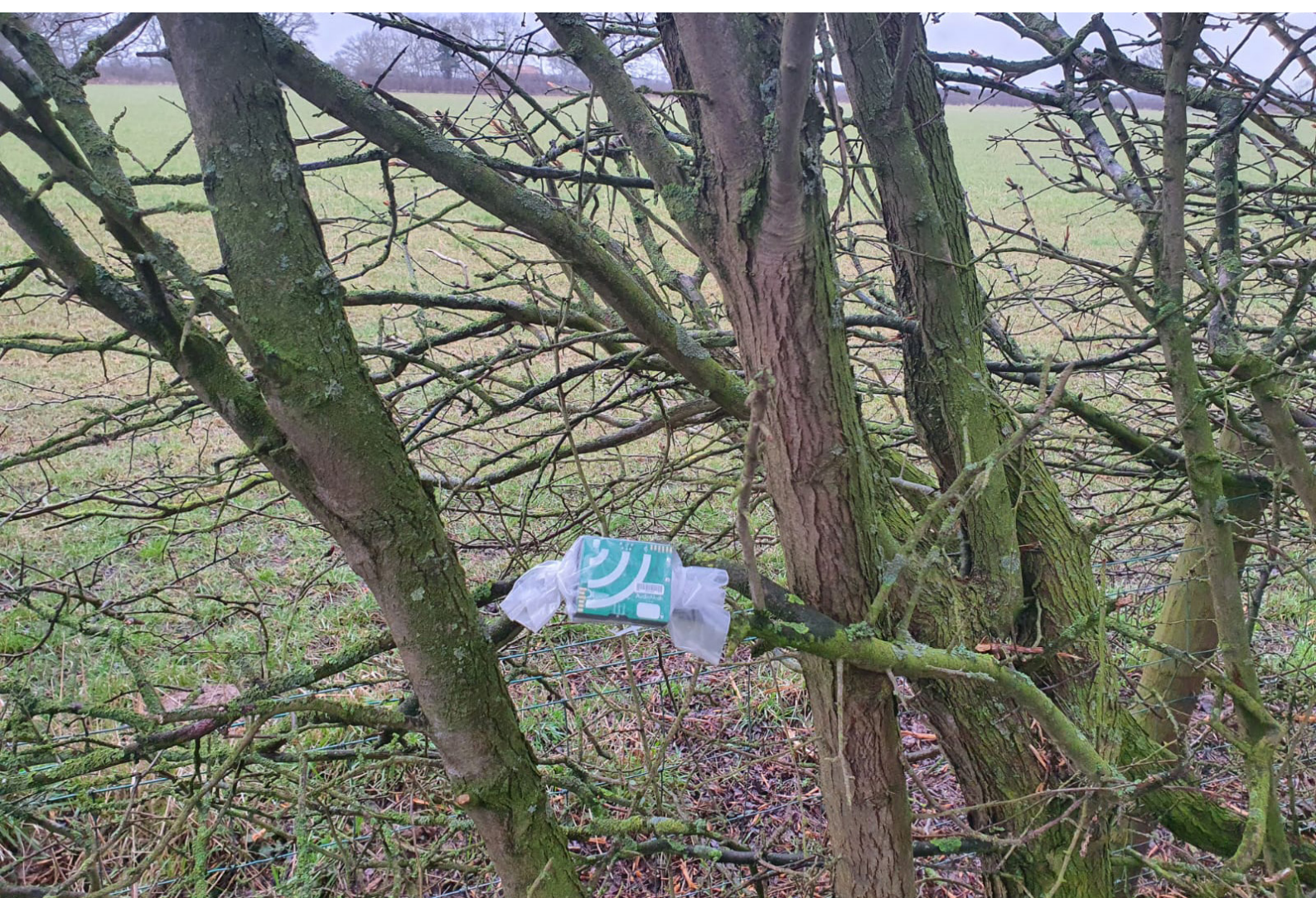
Figure 2.1. Audiomoths are small and relatively cheap, making them readily deployable in a range of locations and with custom-made covers. Credit: Oliver Metcalf.
