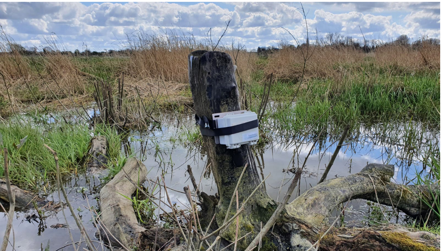
Figure 5.7. A Fronter Labs Bioacoustic Recorder deployed in a Spotted Crake Porzana porzana territory to help monitor this rare, nocturnal, and elusive wetland breeding species. Credit: Oliver Metcalf.
