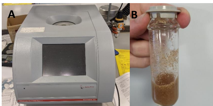
Figure 3.1: A) Anton Paar Monowave 300, B) 30 ml borosilicate reaction vessel
