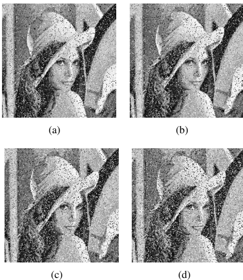
Fig. 13: Decryption of the encrypted images with the noise: k = 0.25 (a); k = 0.5 (b); k = 0.75 (c); k = 1 (d)
