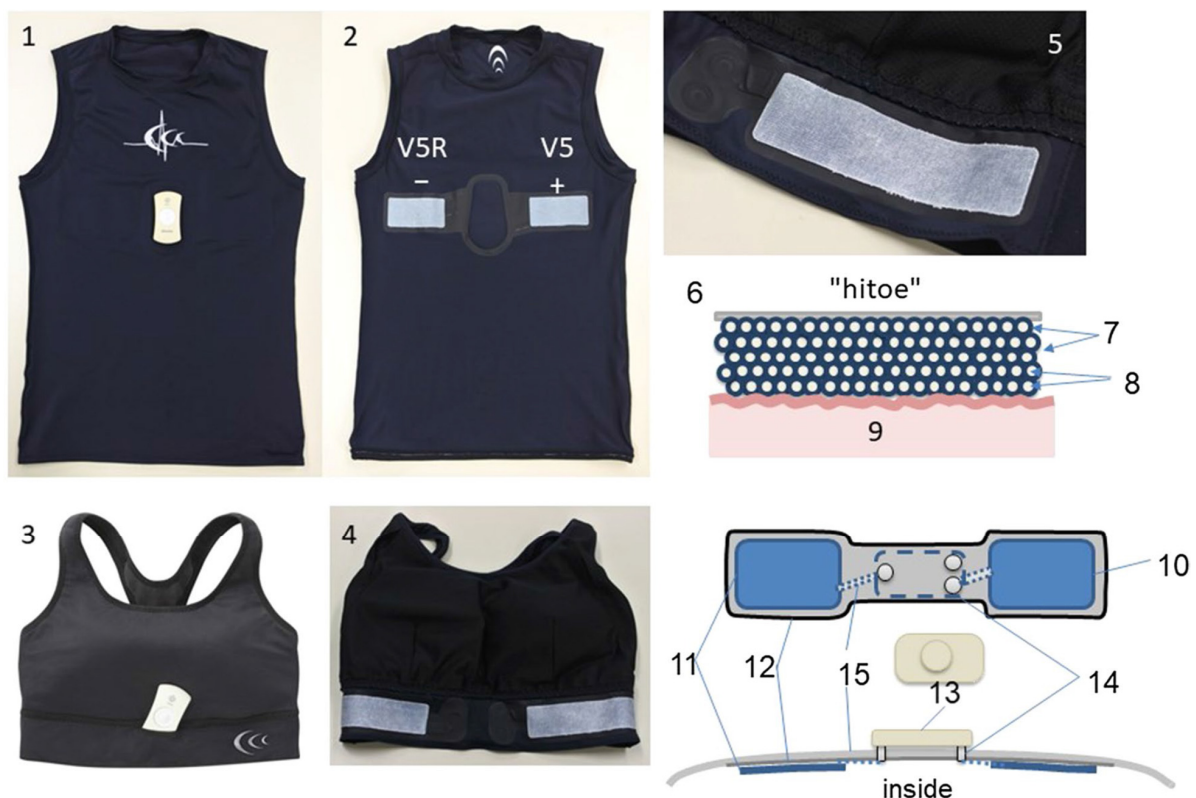
Figure 8. Components of an ECG detecting smart garment. Reprinted from [305].
