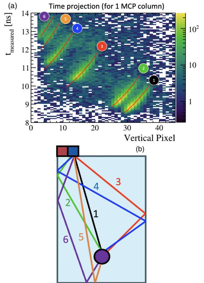
Fig. 6. (a) Photon arrival time on a single horizontal pixel as a function of a pixel in one column. Red lines over the bands show the expected position of the band from simulation. The width of the band can be measured to determine the single-photon time resolution. (b) Six possible paths a photon can take in the radiator, corresponding to the bands shown in (a).
