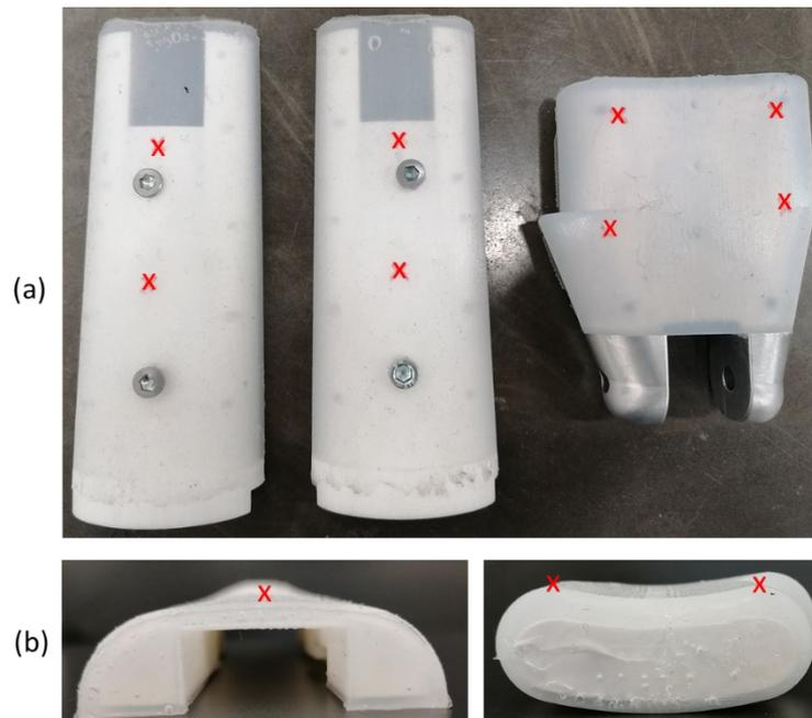
Figure 6-9 Location of the Shore A hardness tests on the compliant hand, conducted before and after testing. (a) top view and (b) front view.
