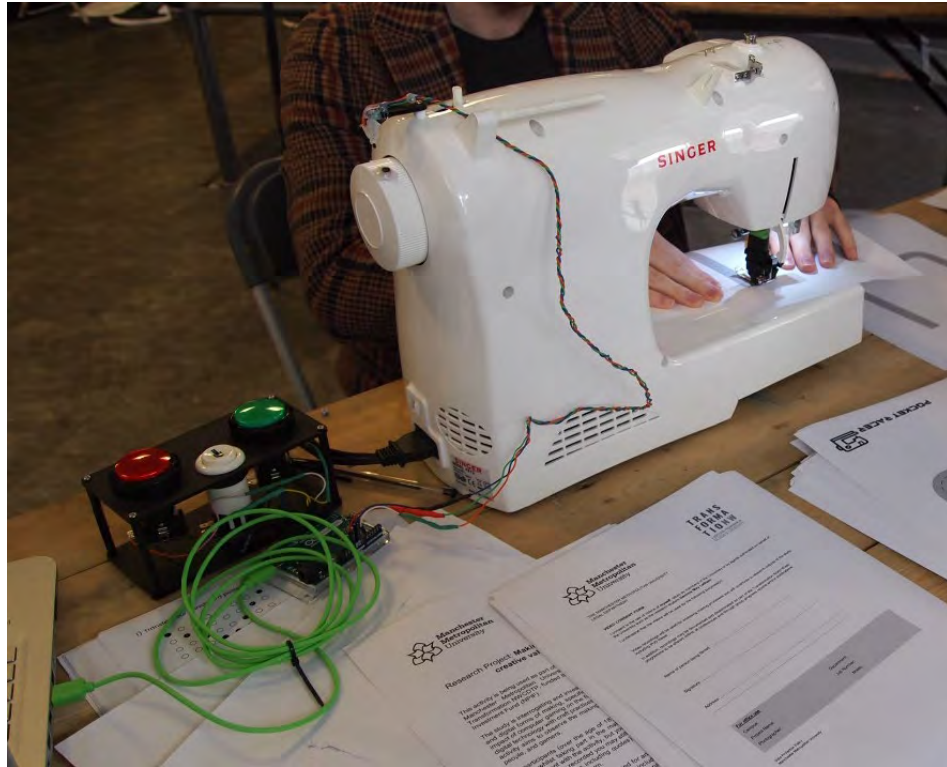
Figure 7.4: Sewing machine with sensor positioned above hand wheel, external Arduino and 'reject'/'accept' buttons
