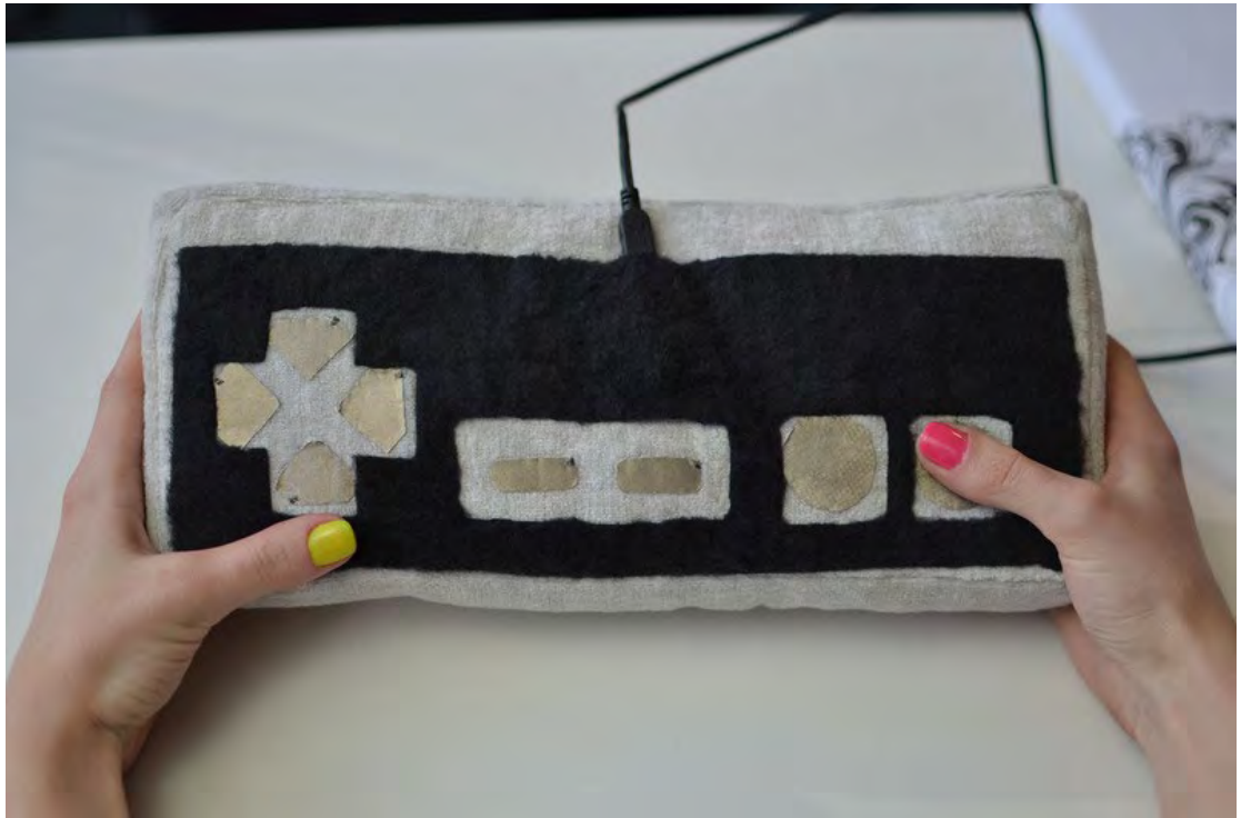
Figure 2.2: Example of a custom-made controller using a Flora board and conductive fabric (Source: Stern, 2013: online)
