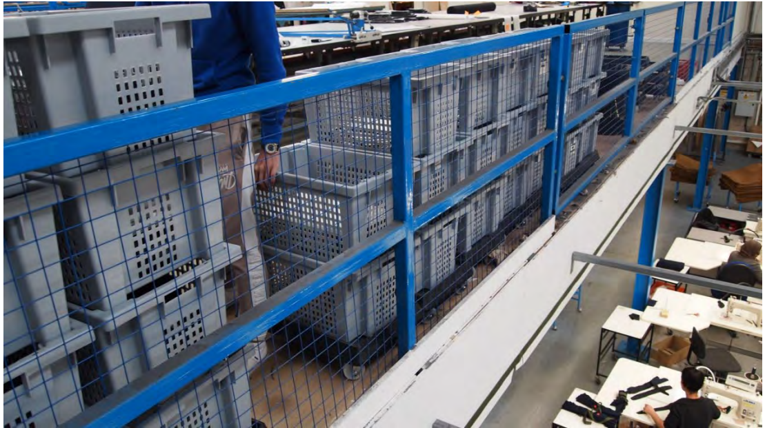
Figure 6.3: Image of mezzanine level with cutting table in the background and crates, where cut batches are sorted, in foreground
