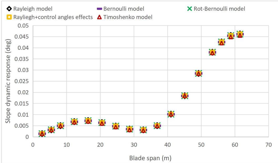
Fig. 19. Edgewise slope distribution along the blade span
