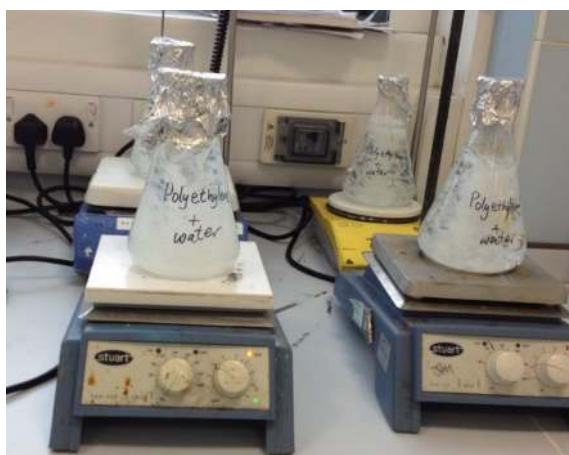
Figure 26: Experimental set-up of migration test 208, 218 undertaken at MMU
