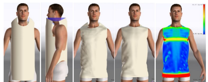
Figure 5. Steps in virtual simulation of clothing
