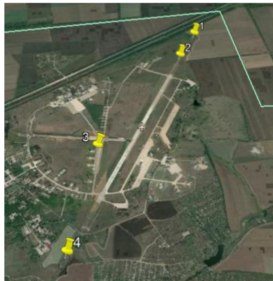
Figure 6. Control points for aircraft noise measurements at Zaporizhzhia International Airport.
