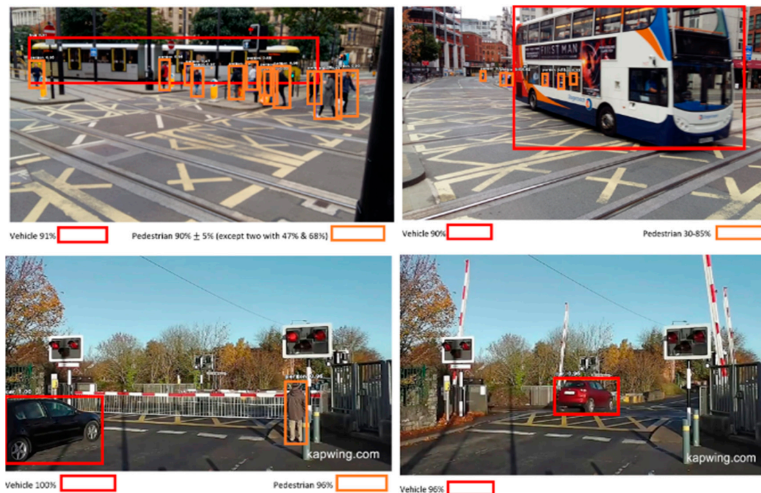
Figure 5. Object detection of multiple objects at two different sites of Level Crossing.
