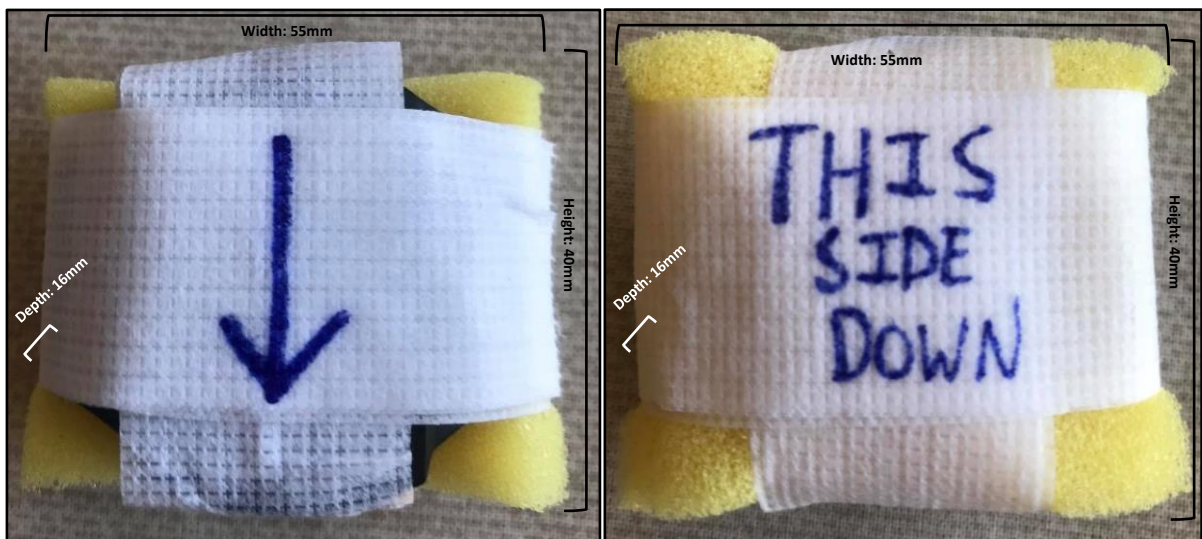
Figure 2.3- Photographic representation of assembled physical behaviour monitoring equipment. From left to right, Anterior view, of assembled GENEActiv device (Note: arrow to remind participant of correct orientation), Posterior View (Note: written instruction to remind participant of correct orientation).
