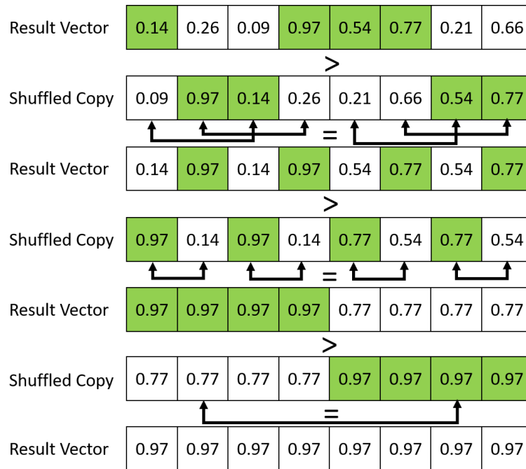
Figure 4.6: A diagram of the parallel reduction technique used to determine the maximum weight in the results vector. This is shown on an 8-wide vector and therefore features one less step than the 16-wide vector implementation.
