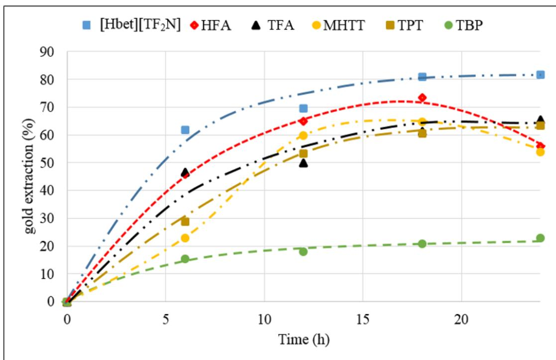
Figure 2 *scCO*<sub>2</sub> extraction of gold with different ligands at 100 bar and 40 °C
