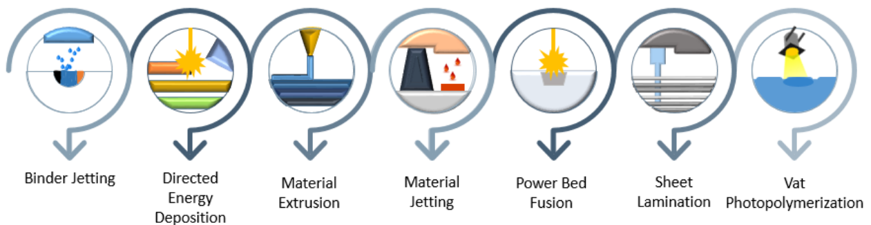
Figure 11. Seven principle categories of 3DP techniques according to the ASTM Standard F2792
