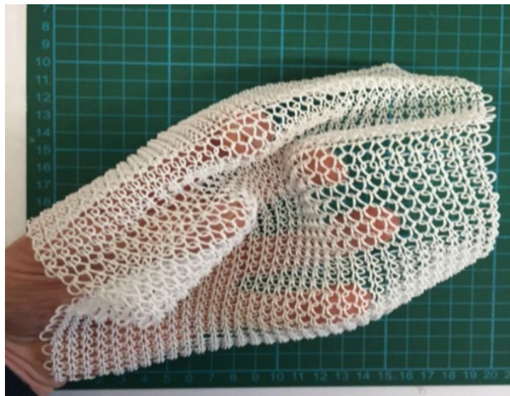
Figure 23. Flexibility of a 3DP weft-knit structure, Reused under the terms of the Creative Commons Attribution 3.0 licence ( https://creativecommons.org/licenses/by/3.0/ ). [26] Copyright 2016, IopScience.
