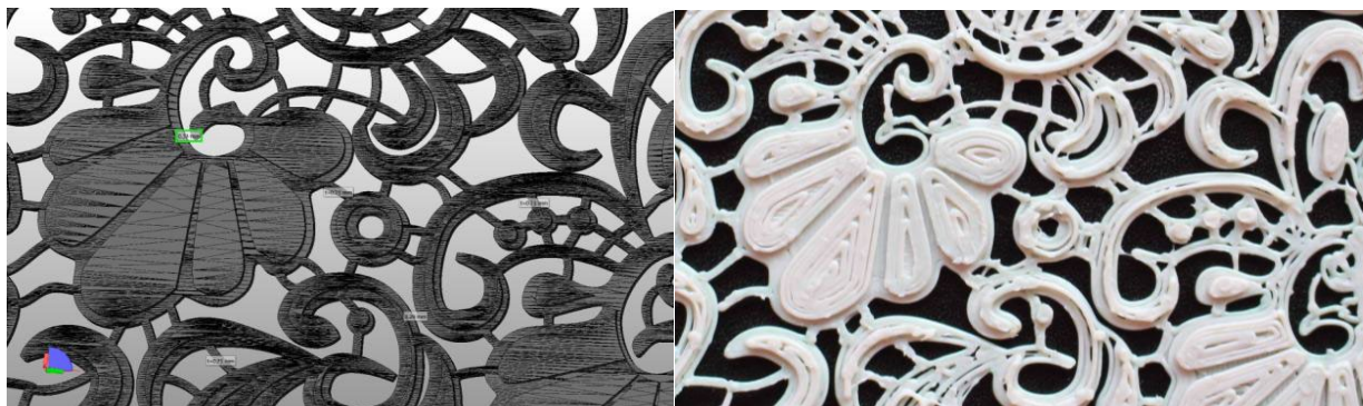
Figure 22. Multi-layer lace pattern, depicted in “netfabb” (left panel), and the resulting 3D print (right panel) - detail dimension ~ 4 cm x 7 cm, Reused under the terms of the Creative Commons Attribution 3.0 licence ( https://creativecommons.org/licenses/by/3.0/ ). [167] Copyright 2014, lopScience.
