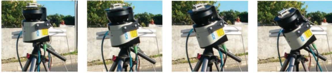
Figure 8A mechanical Laser scanner whose mechanical movement of the system allow the sensor to capture a 3D image.
