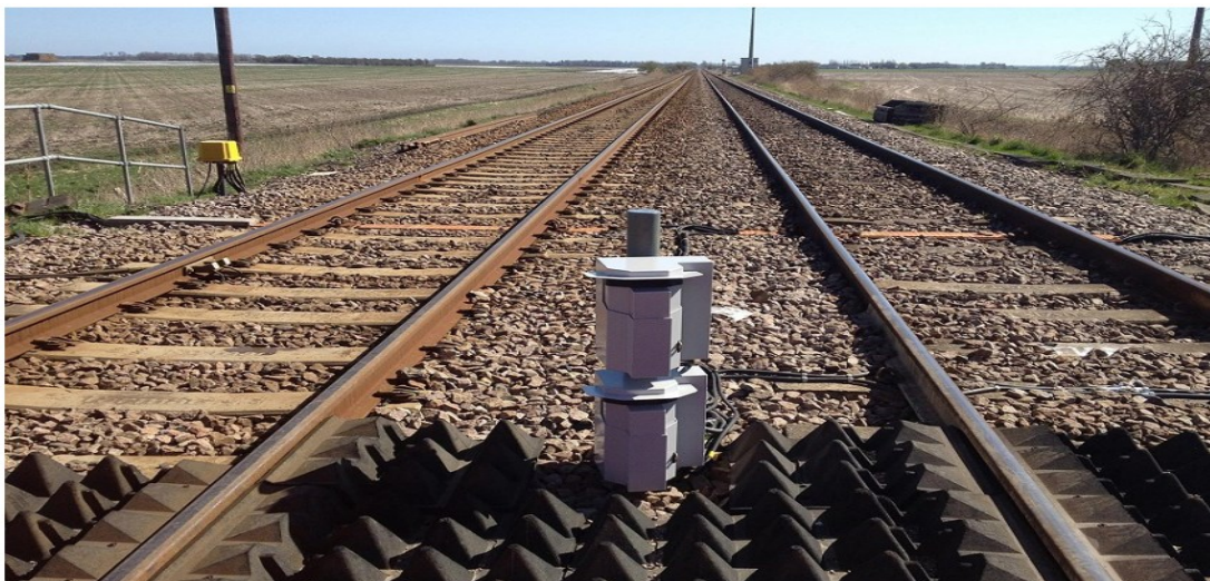
Figure 9LiDAR installed at a Level Crossing site. Picture Courtesy of (Roberts, 2020).
