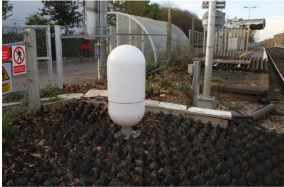
Figure 11A RADAR sensor installed at a Level Crossing site in East Sussex, UK.
