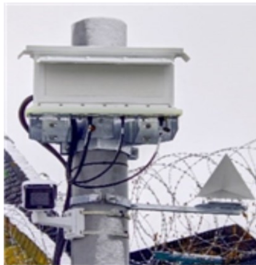
Figure 12 Second Generation Obstacle Detector-OD2. The OD2 is pole mounted RADAR scanner, which is able to replace old RADAR and LiDAR at a Level Crossing site.
