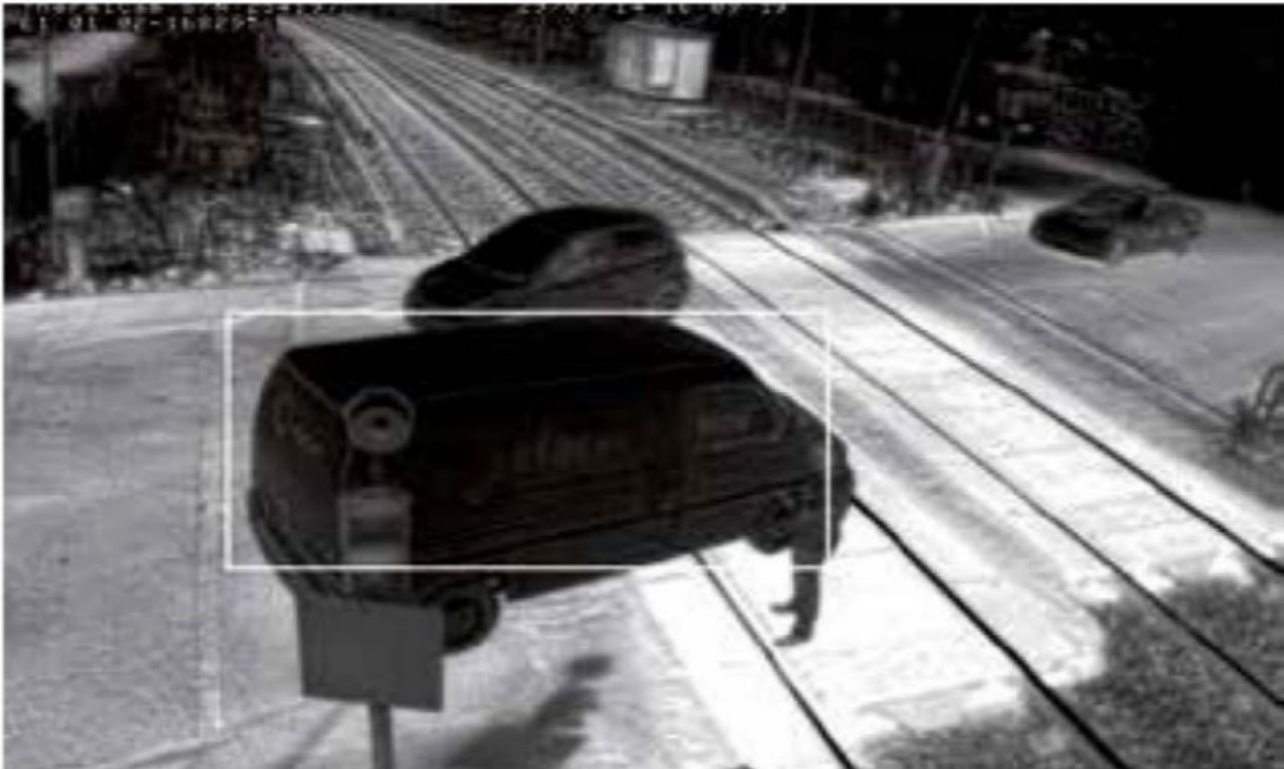
Figure 6 Thermal Imaging at a Level Crossing, where Pedestrian and Vehicle is clearly distinguished.
