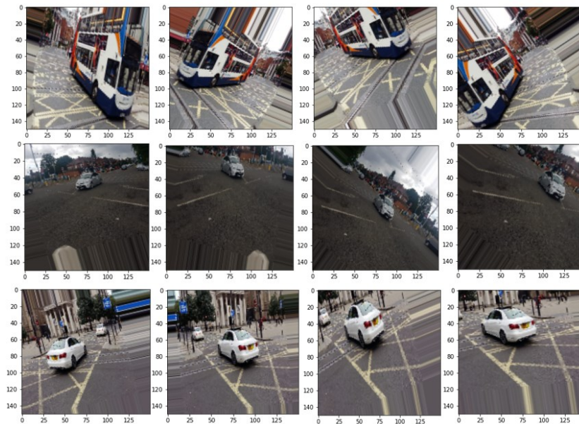
Figure 28 Data Augmentation on three different images from our training dataset. These images have been zoomed, shifted and flipped as shown.
