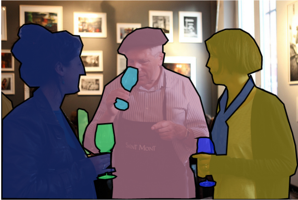
Figure 2.11: Example of an image in MS-COCO with superimposed ground truth. Each instance of an object class is labelled separately. For example, each person in this image is segmented using a different colour. [ https://cocodataset.org/#home ]
