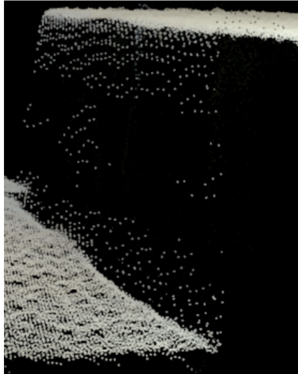
Figure D.5: Flying pixels caused by the Kinect 2 erroneously estimating that the pixels near the edge of the two adjacent objects are at a depth that is halfway between the depth of the objects and that of the background. (Image adapted from: [13])
