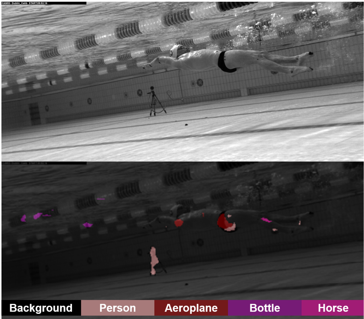
Figure 2.3: DeepLab v3+ is the most sophisticated algorithm for silhouette extraction available to date. However, even it does not perform well on images that come from a domain on which it was not trained—for examples, on images of underwater swimmers. (Image created by the author)
