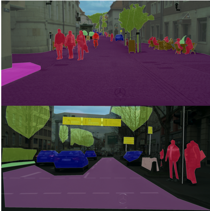
Figure 2.12: Top: example of a finely-labelled image in Cityscapes. Bottom: examples of a coarsely-labelled image in Cityscapes. [ https://www.cityscapes-dataset.com/ ]
