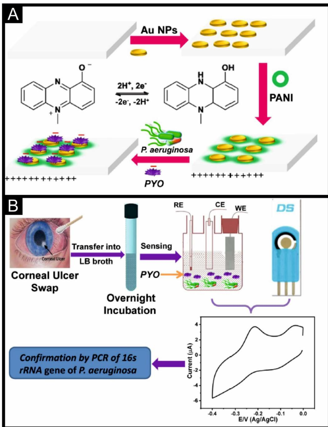
**Fig. 4.** (A) Schematic diagram of the PANI/AuNPs/ITO SPE fabrication and the PANI-PYO interaction. (B) Schematic representation of the electrochemical sensing of *P. aeruginosa* using the SPE sensors and an example of its electrochemical signal. Adapted and reprinted with permission from [106].
