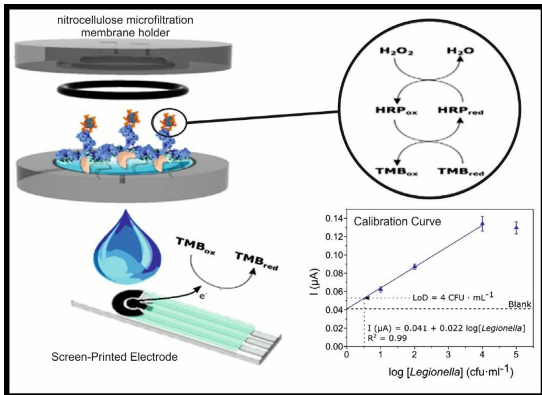
**Fig. 5.** Schematic diagram of the microfiltration, immunoassay, screen-printed electrode platform and calibration curve for the determination of *Legionella pneumophila* in drinking water. Adapted and reprinted with permission from [109].
