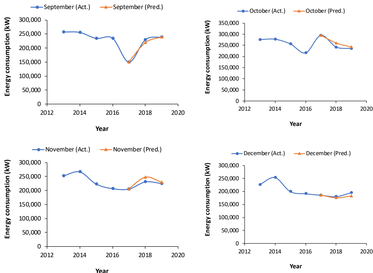
Figure 11. Energy consumptions prediction on a monthly basis for the year 2018 and 2019 using the MLA. (e.g., November (Act.) and November (Pred.).)
