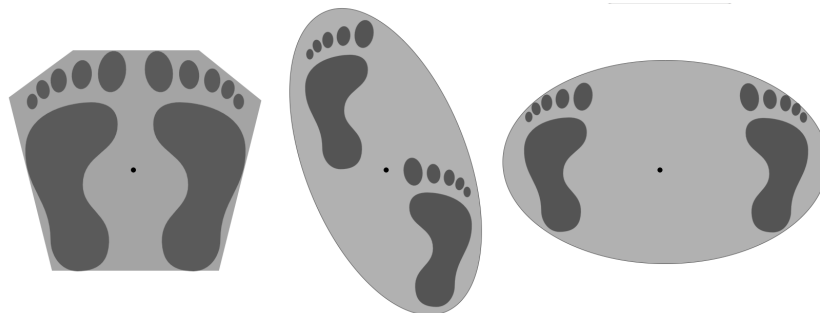
Figure 2.1: CoP in relation to the BoS. the CoP is marked by a black dot This figure shows three possible BoS (shaded grey), and the associated CoP (shown as a black dot). The first two are narrow stances, quiet standing and semi-tandem, repetitively. The third is a wide version of quiet standing (feet shoulder width apart).
