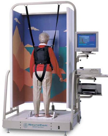
Figure 2.3: SMART Balance Master: The SMART Balance Master, is one of the few devices used in the clinical assessment of balance. However, it widescale adoption is restricted by its size and cost.
