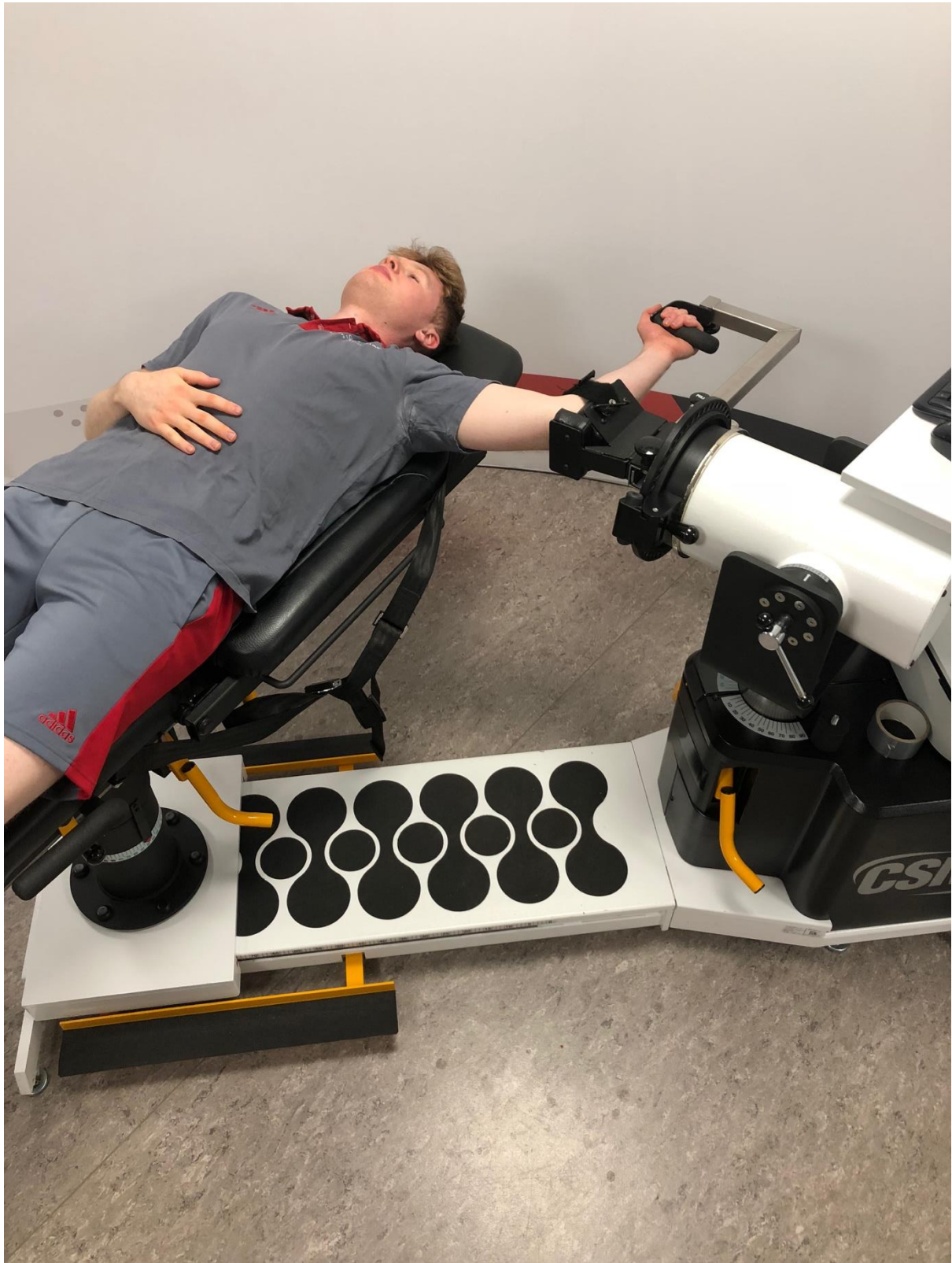
Figure 2 Setup for Isokinetic Shoulder Internal and External Using an Isokinetic Dynamometer
