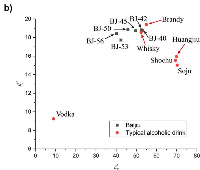
**Fig. 6.** Comparison of the resonant responses and dielectric properties of the baijiu and other alcohol samples: (a)  $f_r$ - $Q$  diagram; (b)  $\epsilon'_r$ - $\epsilon''_r$  diagram.
