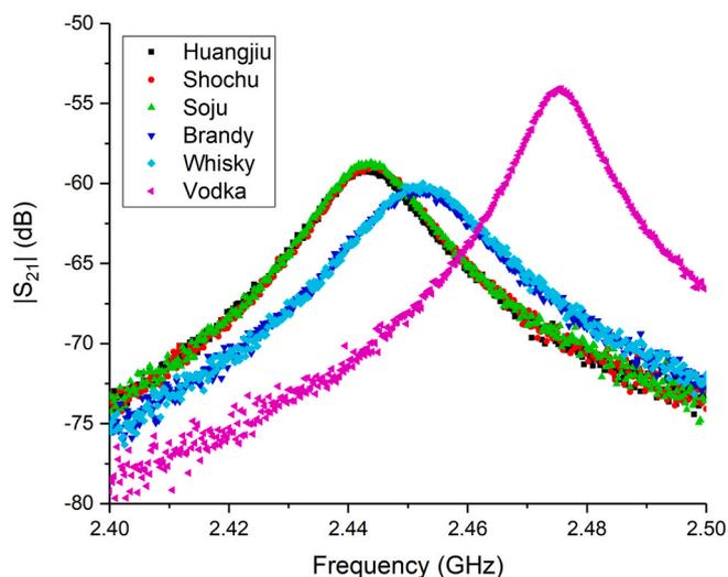
Fig. 5. Signal responses of six other alcohol samples.
