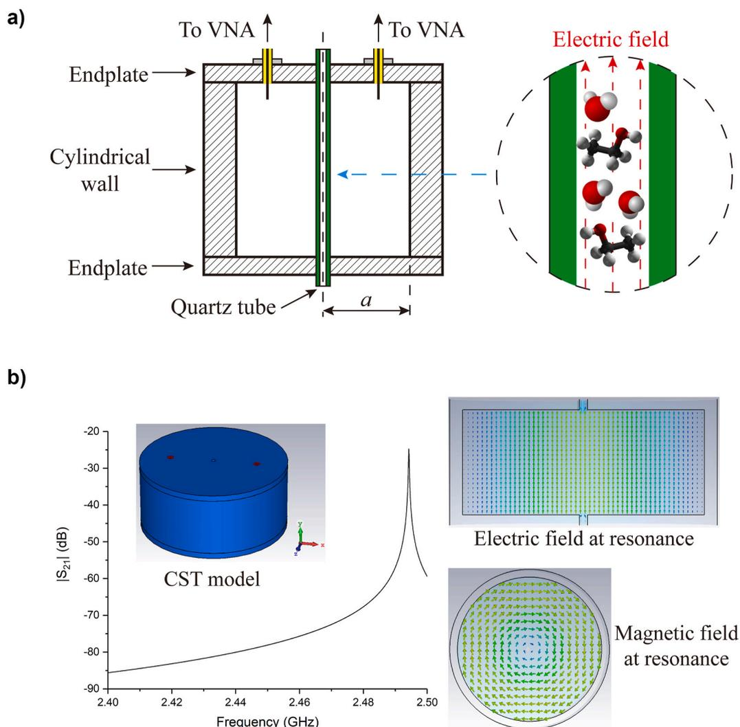
**Fig. 1.**  $TM_{010}$  mode cylindrical cavity resonator developed: (a) cross section; (b) electromagnetic simulation model and results including the frequency responses and the field distributions at resonance.
