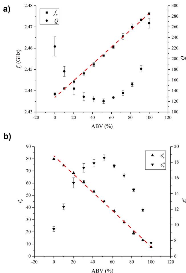
**Fig. 8.** Variations of the resonant parameters and dielectric properties of the ethanol-water mixtures with respect to ABV (error bars represent the deviations of four replicates): (a)  $f_r$  and  $Q$ ; (b)  $\epsilon_r'$  and  $\epsilon_r''$
