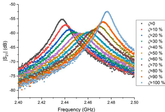
**Fig. 7.** Resonant responses of the ethanol-water mixtures.
