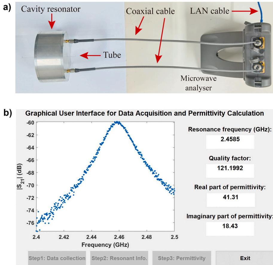
Fig. 2. Experimental setup for the evaluation of liquid samples using the microwave resonator sensor: (a) photograph; (b) graphical user interface for easy data acquisition and processing.
