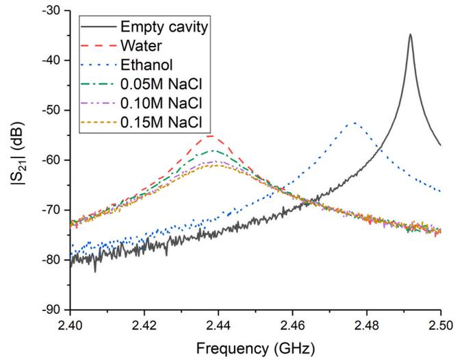
Fig. 3. Signal responses of the empty cavity and standard liquids.
