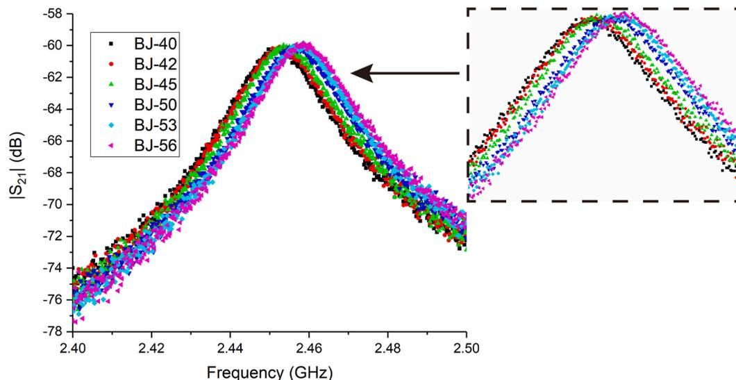
Fig. 4. Resonance curves of the baijiu samples.
