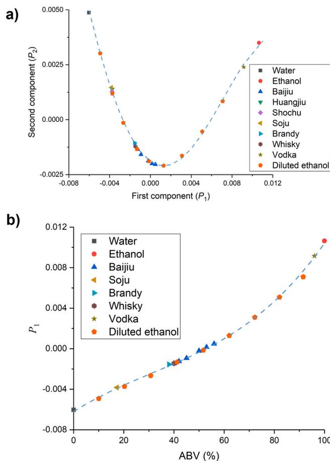
**Fig. 9.** PCA results from the resonant responses of all the samples measured: (a) score plot of the first component values versus the second component values; (b) variation of the first component value with respect to ABV.
