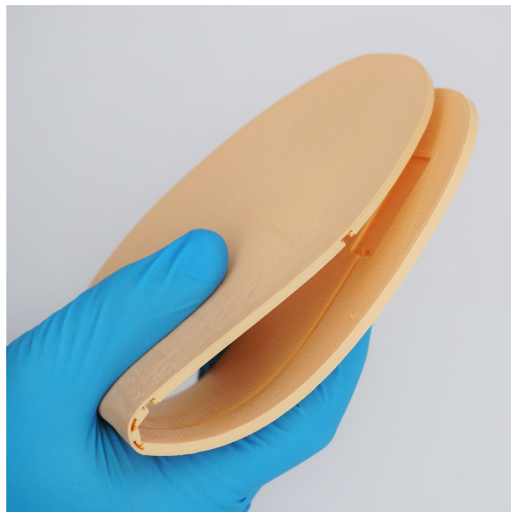
Figure 2. Demonstration of the flexibility of the 3D-printed insoles used in this study.
