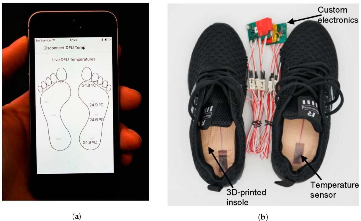
**Figure 3.** New wearable sensor insole system developed in this work for the continuous monitoring of plantar foot temperatures. (a) The iPhone app used for real-time visualisation and logging of data; (b) The smart insole system used by participants with the devices fitted inside shoes.
