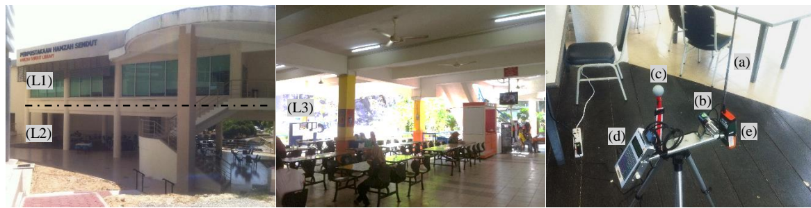
Figure 1. Locations and instruments. (L1) 24-hour reading room. (L2) Semi-outdoor reading area of the library. (L3) Dining hall of RESTU and SAUJANA hostels. (a) air velocity . (b) air temperature and humidity . (c) globe temperature. (d & e) data logger.
